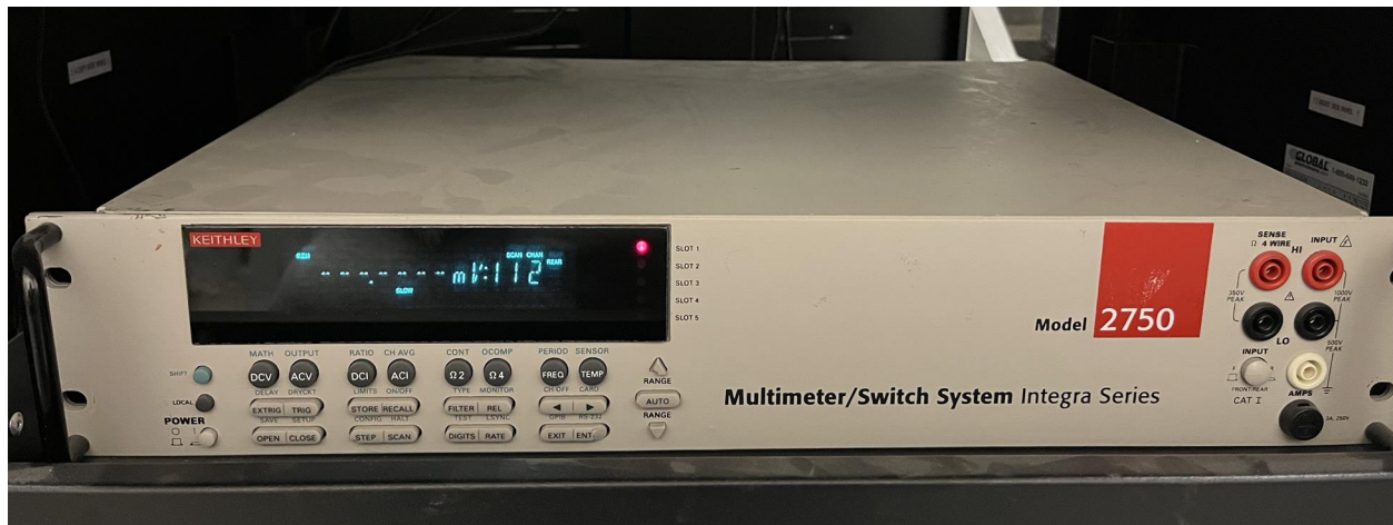
Figure 4. Keithley Multimeter / Switch System
