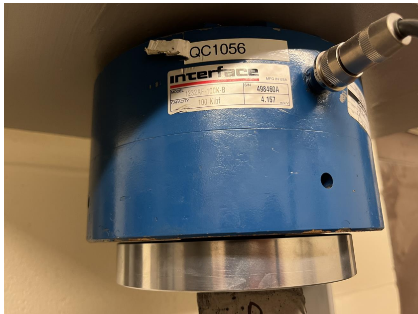
Figure 3. 100-kip load cell placed at top of creep frame
