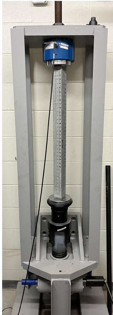
Figure 11. Test specimen loaded into creep frame
