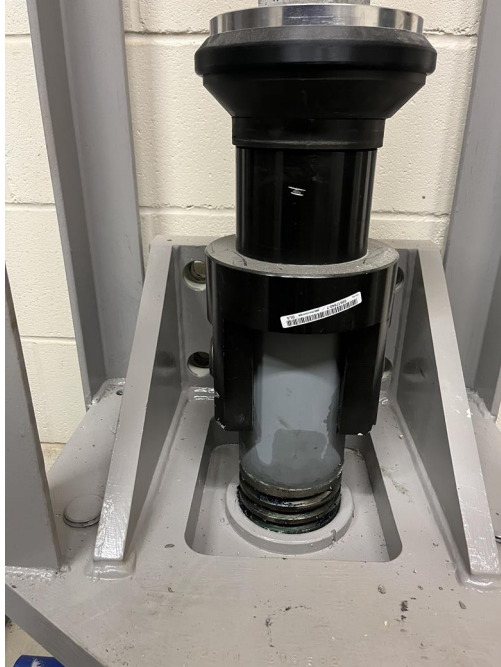
Figure 2. Screw driven loading jack
