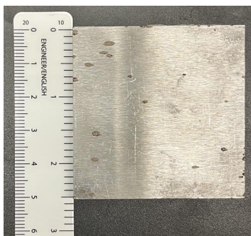
Figure 10. 2.5" by 2.5" by 1/4" steel cap plate
