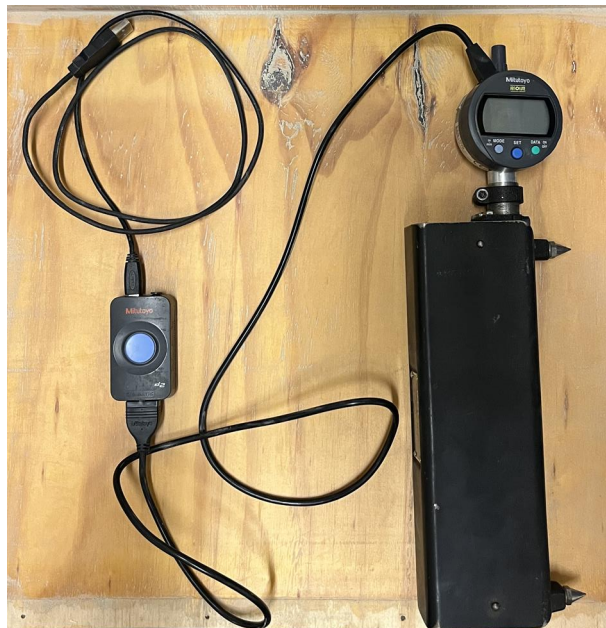
Figure 6. Whittemore strain gauge with Mitutoyo input tool
