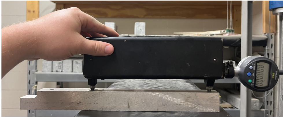
Figure 13. Zero test performed before taking measurements
