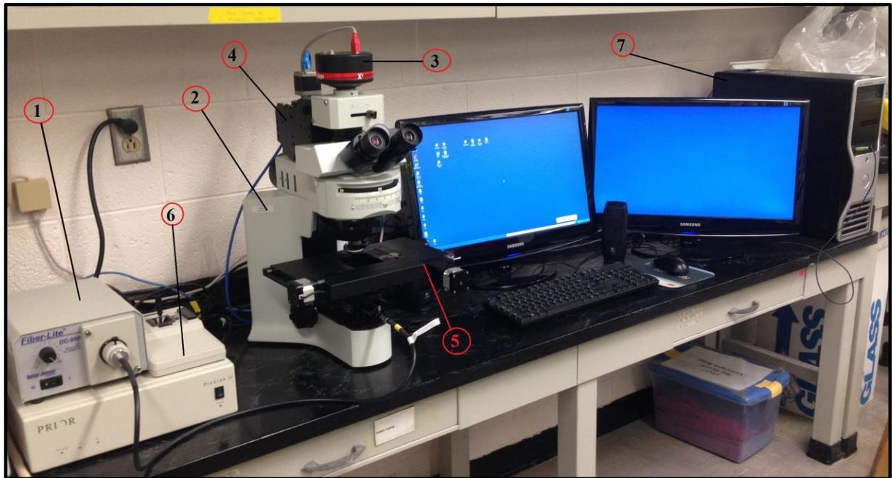
**Figure 5.2 CytoViva® Hyperspectral Imaging Microscope System. 1: Halogen light source; 2: Optical microscope; 3: Optical Camera; 4: VNIR spectrophotometer; 5: Motorized stage; 6: Controller for stage; 7: Computer**
