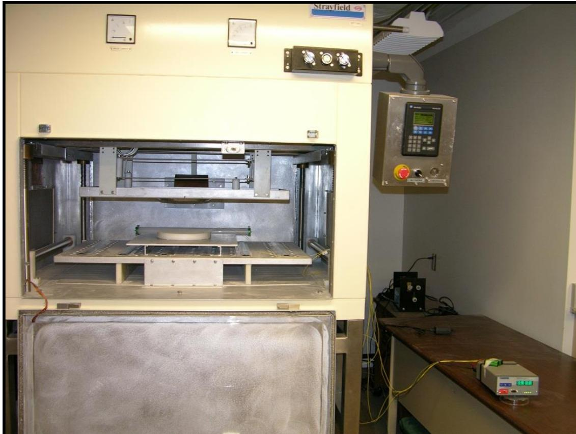
**Figure 4.3** Radio frequency dielectric heating unit
