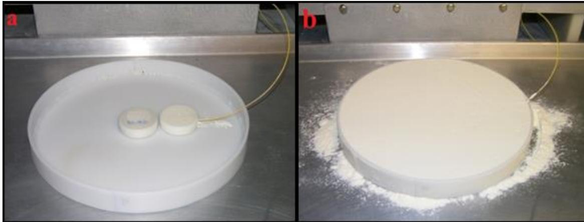
**Figure 4.2 Inoculated and non-inoculated (connected with fiber-optic probe) nonfat dry milk in sealed containers in high-density polyethylene tray for radio frequency dielectric heating: a) before covering with non-inoculated nonfat dry milk; b) after covering with non-inoculated nonfat dry milk**
