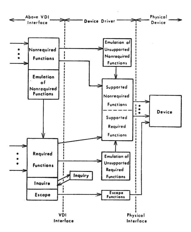
Figure 2.4 Virtual Device Interface Model
