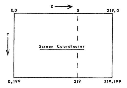
Figure 3.2 - Display Screen Characteristics
