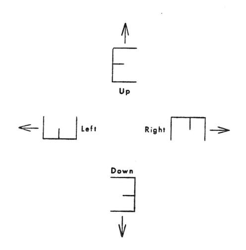
Figure 3.7 Illustration of Text Path Vector Concept
