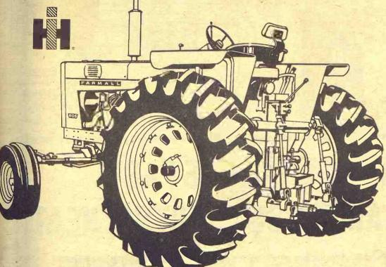
Unlike some big tractors, the Farmall® 806 and 1206 Turbo are engineered for new high-traction 38-inch tires.
