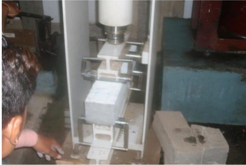
Figure 5: Testing of Flexural Strength Test Specimen
