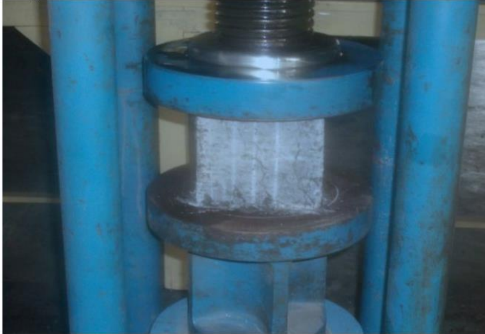
Figure 4: Testing of Compressive Strength Test Specimen
