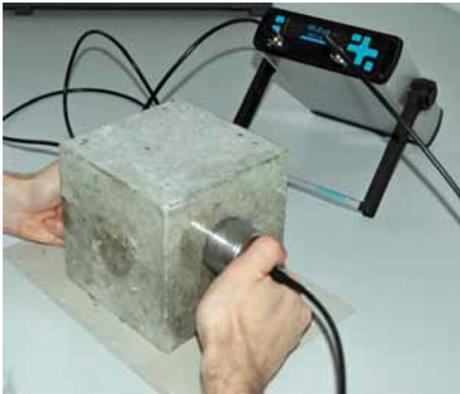
Figure 7: Testing for Ultrasonic Pulse Velocity Test
