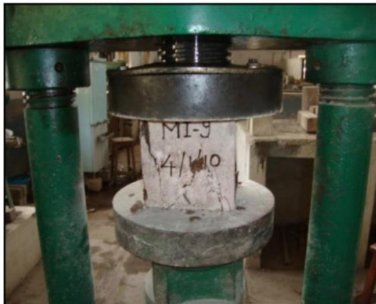
Figure 6: Testing for Split Tensile Strength Test Specimen
