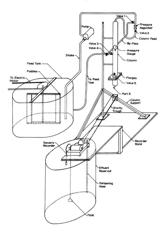
for mixing, but it also made the control of the initial inlet water much easier. This aided in the prevention of surging across the filter which was necessary to allow the initial cake to deposit uniformly. Entering the water first at this point also limited undue stresses on the cloth. The small draw-off valve, 4, was used to obtain samples of the influent. It was thought that this location would allow very representative samples of the water going through the filter to be taken.
