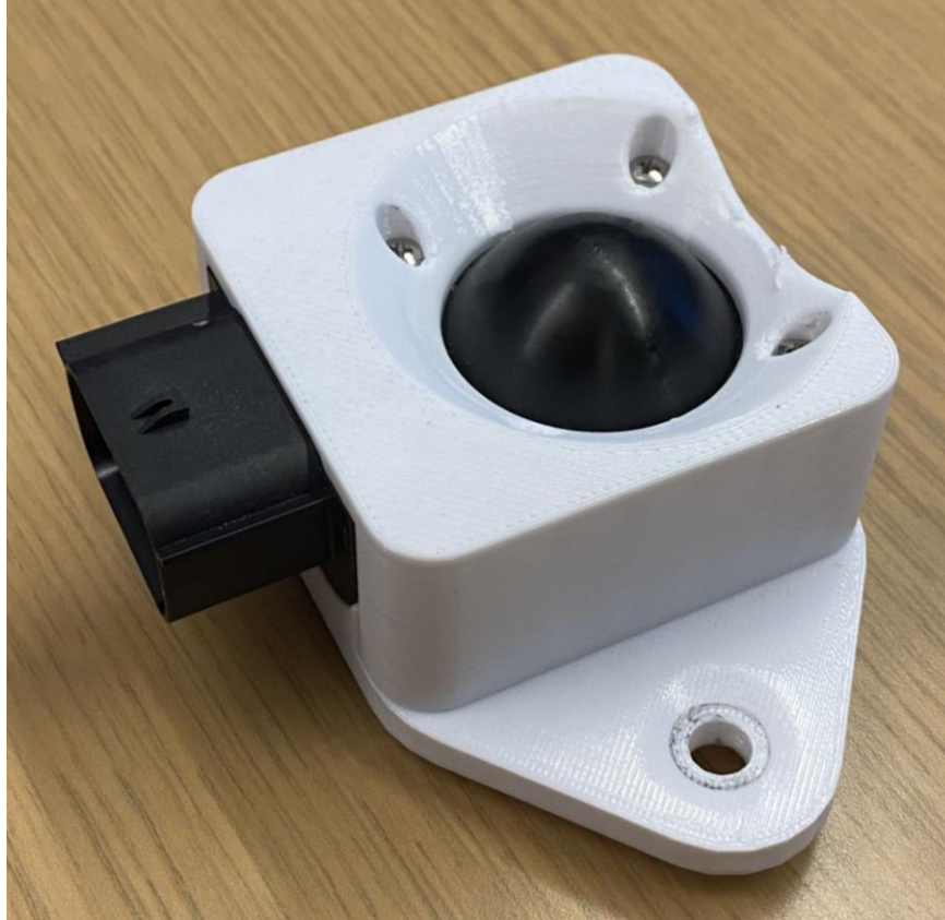
Figure 2.4. Mechanical housing and focusing lens for AGR 120.
