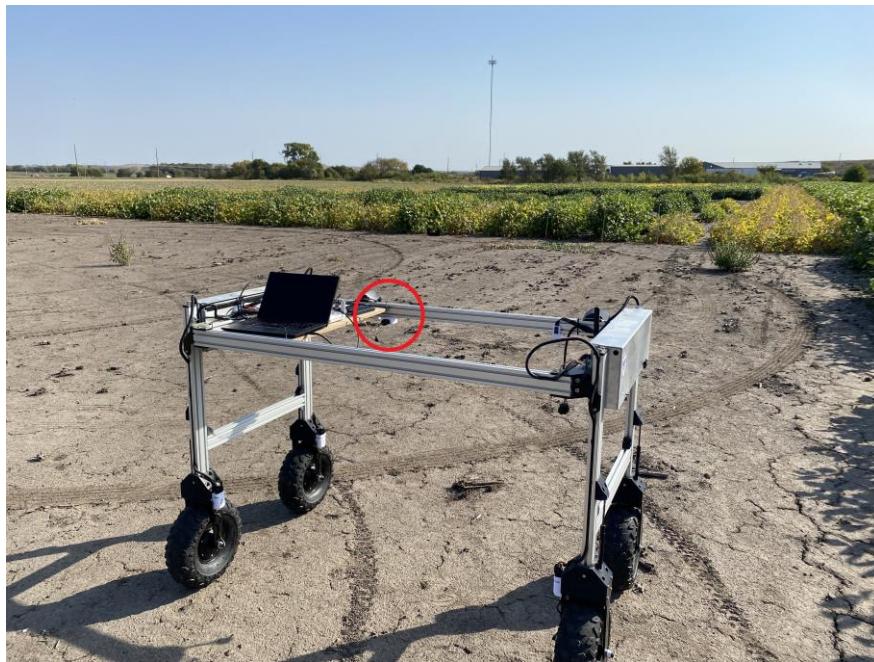
Figure 4.1. Field test setup with AGR 120 (circled in red) attached to rover.
