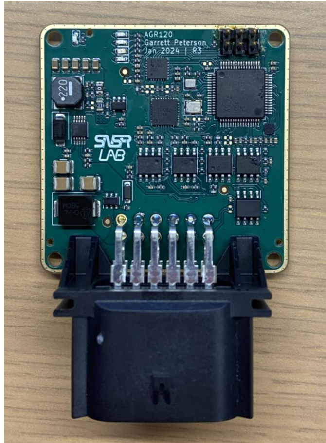
Figure 2.3. Assembled AGR 120 PCB.
