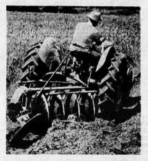
be set shallow for summer-fallow for effective weed control at stepped-up speeds. High frame clearance minimizes "trashing up" in turning under cover crops. The tiller's large earth-moving capacity makes it useful in economical terrace building and gully filling.
