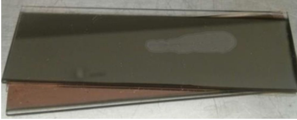
Figure 4.11: NiCr/Cu coated glass with a pure In diffusion bond formed at 350 °C over 24 hr 28 . Over this period, indium diffused through the entire 400 nm film.
