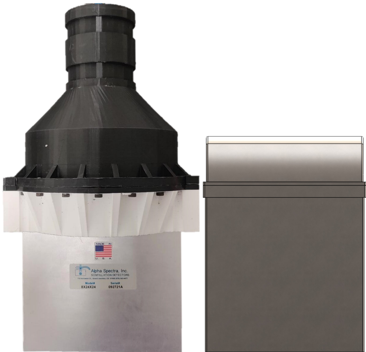
Figure 3.31: Size comparison of spectrometers using 50.8 \times 152.4 \times 152.4 mm scintillator crystals. On the left, a 127 mm PMT is shown, while a model of the Catoptric PMT paired to the crystal housing is displayed on the right.
