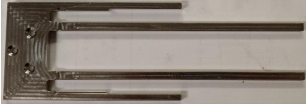
Figure 5.6: The end-effector mounted the axial manipulator prior to polishing. The fork design enables stable transfer of the window, dynodes, and PMT envelope.
