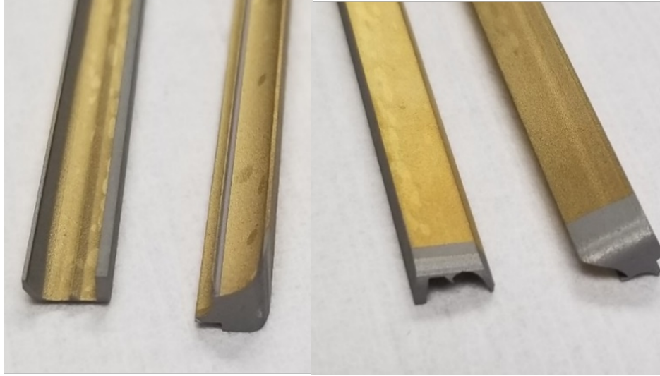
Figure 4.12: The metalized aluminum wire-EDM dynodes. The metalized surface provided low resistivity across the electrode but could not maintain isolation between electrodes.
