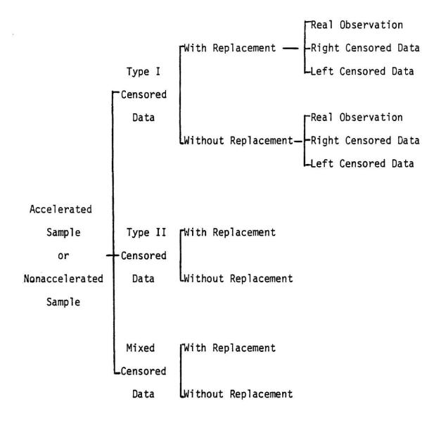
Figure 1. Different forms of sampling that may arise in life testing.
