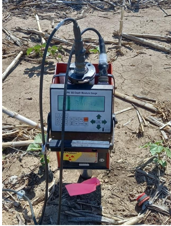
Fig. 3: Picture of a CPN 503 Depth Moisture Gauge set on top of the access tube
