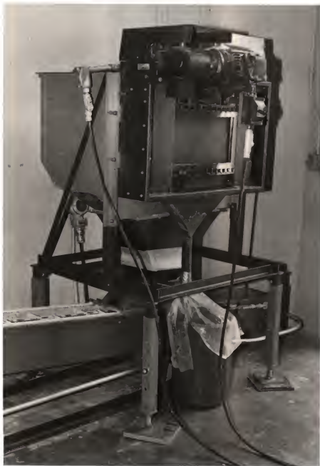
Figure 7. Gamet Automatic Sampler situated at the inlet of the conveyor.
