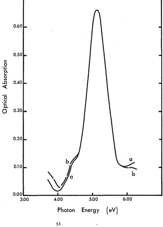
Optical absorption spectra of irradiated LiF measured with [011] polarized light at 90°K before and after an optical bleach with [011] polarized light at 90°K. Curve (a) is the optical absorption spectrum before the bleach. Curve (b) is the optical absorption spectrum after a 90 min. bleach at 244 nm. Absorbed Dose - 0.12 Mrad
