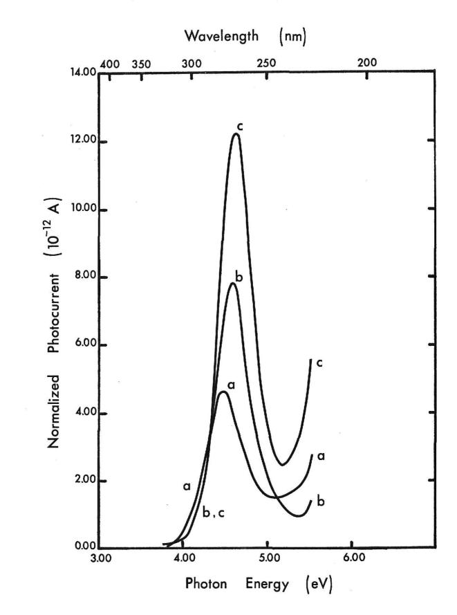
Temperature dependence of the peak position of the 4.46 eV, at  $300^{\circ}\text{K}$ , photocurrent peak
