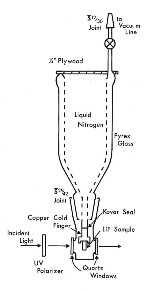
Experimental arrangement used in determining the effect of optical bleaching on the optical-absorption spectra.
