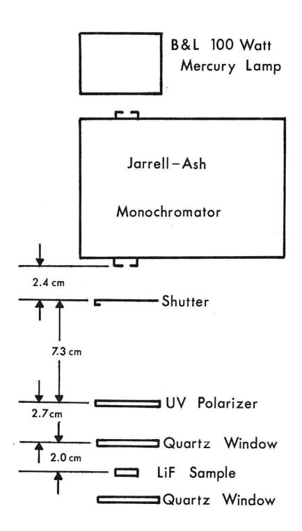
as the bleaching source. The Jarrell-Ash monochromator has a dispersion of 1.6 nm/mm in the ultraviolet. A one millimeter exit slit was used giving a bandpass of 1.6 nm. A linear polarizer made by Polacoat Inc. was employed to polarize the light from the monochromator when bleaching with [011] polarized light. The spectral range of the polarizer was 240 nm to 400 nm.
