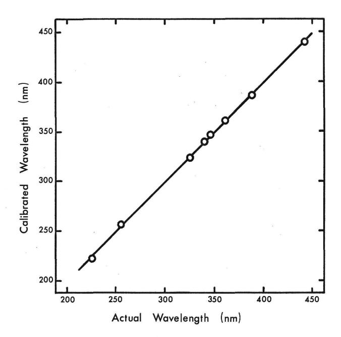
Wavelength calibration curve for the Bausch and Lomb monochromator. The solid line represents a least-squares fit to the experimental data.
