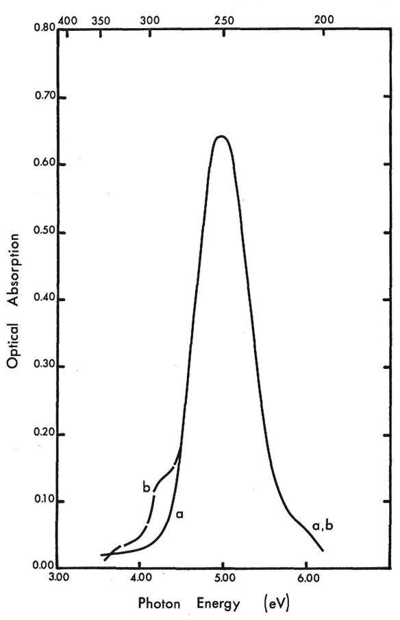
exhibits dichroic behavior for the two polarizations with the optical absorption being larger for the [011] polarized light. Figure 12 shows the dichroic optical absorption of the Y center at 90°K. Figure 12a is the absorption spectrum measured with [011] polarized light and Fig. 12b is the absorption spectrum measured with [011] polarized light.
