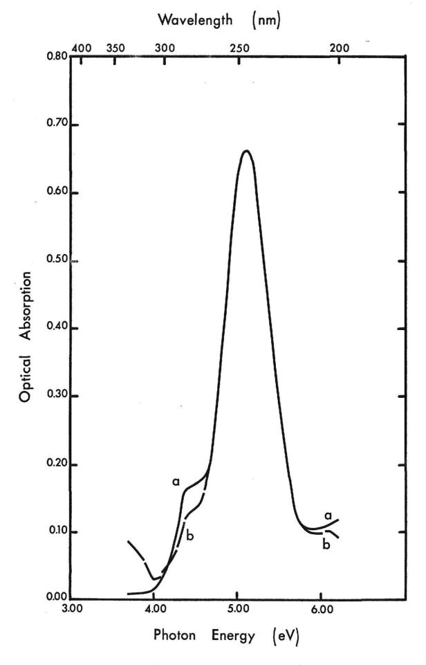
optical bleach with [011] polarized light is the same as that observed for unpolarized light. The dichroism of the Y center has disappeared and the Y center optical absorption for the two polarizations is equal after the optical bleach.
