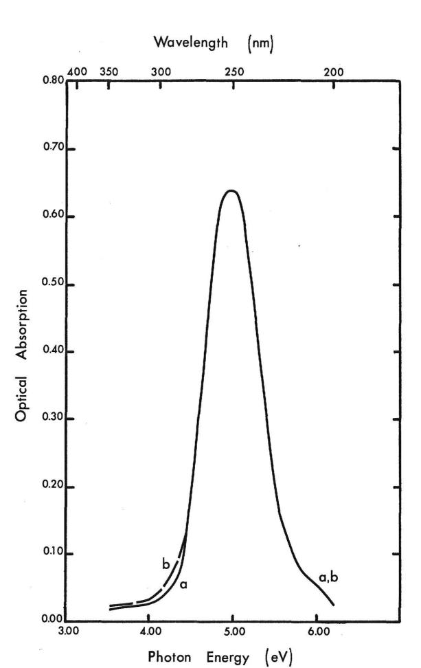
Optical absorption spectra of irradiated LiF measured with [011] polarized light at 300°K before and after an optical bleach with unpolarized light at 300°K. Curve (a) is the optical absorption spectrum before the bleach. Curve (b) is the optical absorption spectrum after a 930 min. bleach at 254 nm. Absorbed Dose - 0.12 Mrad
