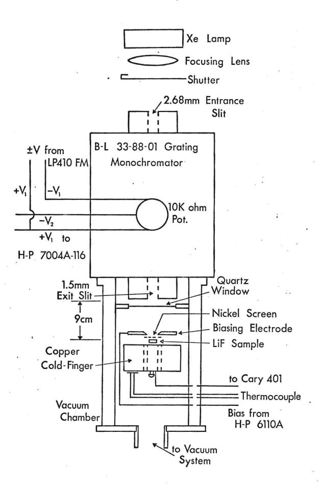
Side view of the vacuum chamber, cold finger and sample holder used in the photoconductivity
