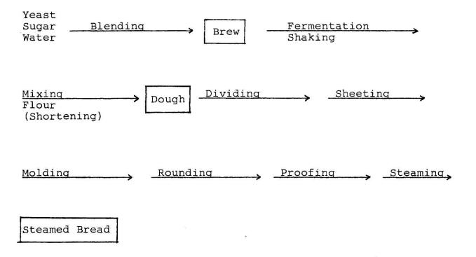
Figure 3. Processing of Steamed Bread - Liquid Ferment System (without flour)
