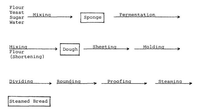
Figure 2. Processing of Steamed Bread - Additional Sheeting Method
