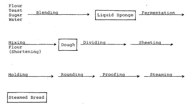
Figure 4. Processing of Steamed Bread - Liquid Ferment System (with flour)
