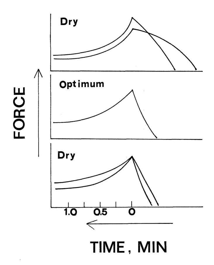
as well as the relaxation changes that occur under given stress. The flow properties, due to liquid bridging, are reduced and the compacted particles demonstrate more solid properties.
