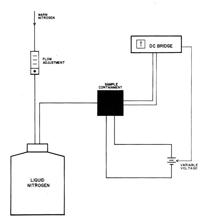
Once again the cell was allowed to come to equilibrium. The stability of the temperature in this case was  $\pm 0.1^{\circ}\text{C}$ .
