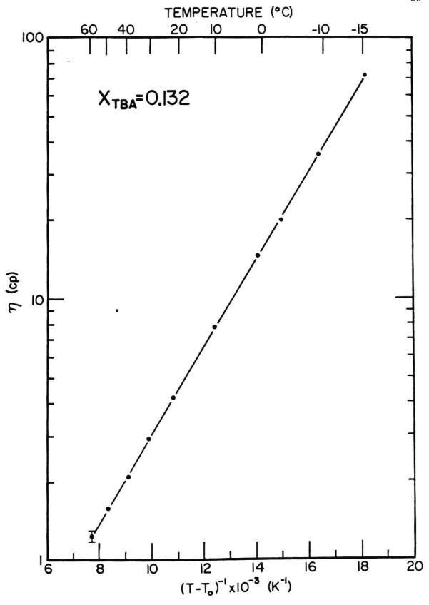
Figure 5-8 VISCOSITY DATA FOR  $X_{TBA} = 0.152$  The line corresponds to the values of  $\eta$  determined by the Vogel-Tammann-Fulcher equation with the best fit parameters.
