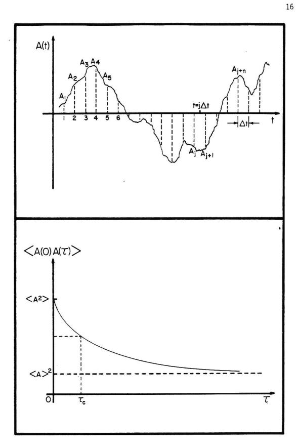
Notice that the time scale in Fig. (3-2) has been divided into intervals of length  $\Delta t$ . This digitizes A(t) so that  $A_j$  denotes the average value of A(t) over the interval  $t=j\Delta t$  to  $t=(j+1)\Delta t$  and likewise  $A_{j+m}$  denotes the average value of A(t) over the interval  $t=(j+m)\Delta t$  to  $t=(j+m+1)\Delta t$ . Under this procedure the correlation function can be approximated by changing the integral to a summation,
