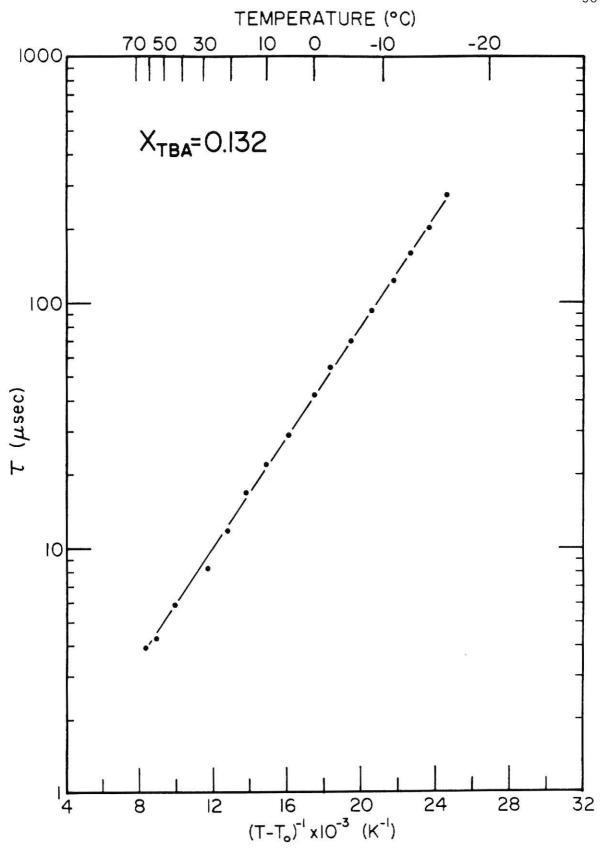
Figure 5-3 CORRELATION TIME DATA FOR X  $_{TBA}$  = 0.152 The line corresponds to value of  $\tau_{_{\scriptsize C}}$  determined by the Vogel-Tammann-Fulcher equation with the best fit parameters.
