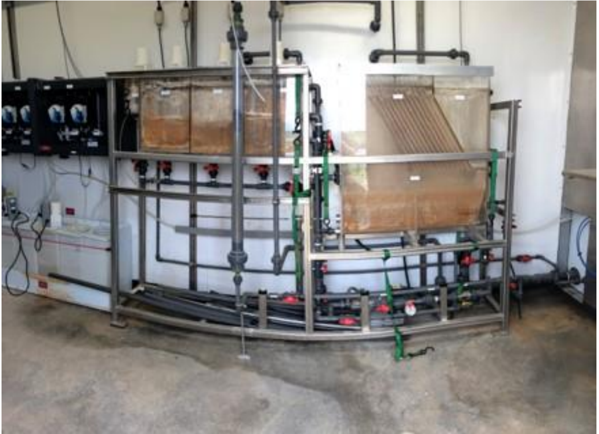
Figure B.4 Coagulation-Flocculation-Sedimentation Process
