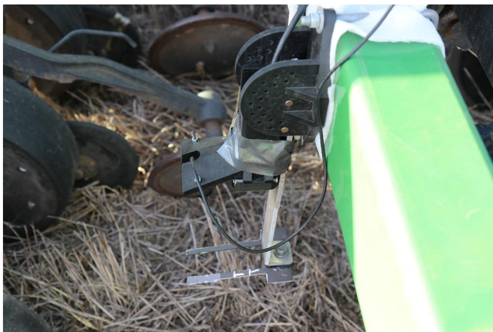
Figure 2.4. Camera inside the 3D-printed mount, fitted to the air-seeder's frame
