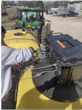
Figure 3.6. DAQ box mounting on the planter (left), accelerometers mounted on the row unit (middle), and hydraulic pressure transducers (right).
