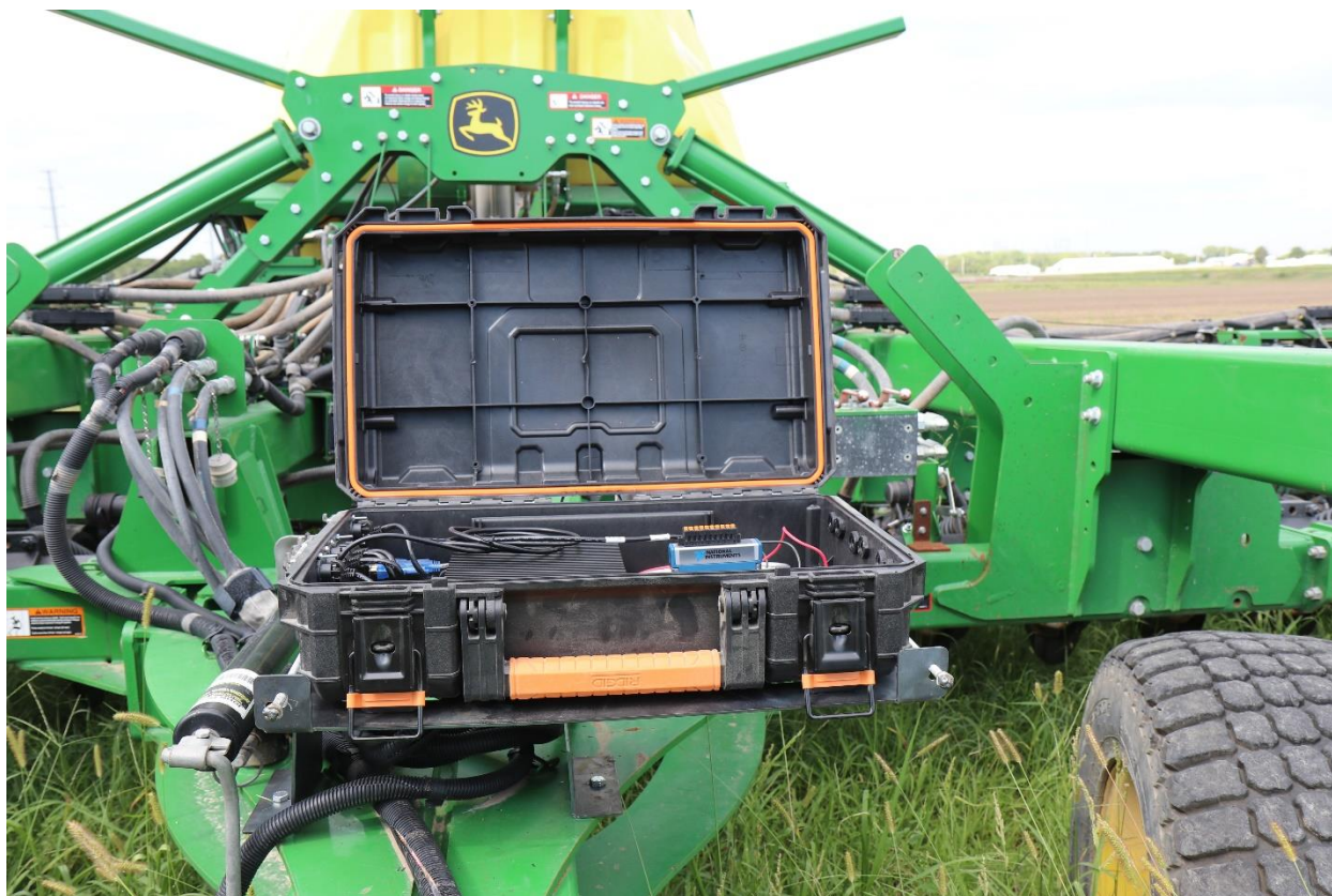
Figure 2.7. DAQ box sitting on the tailor-made mount fitted on the air-seeder
