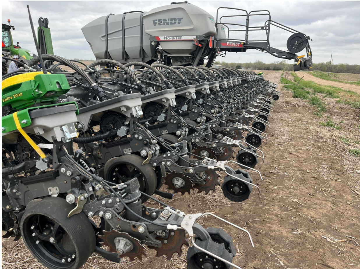
Figure 3.7. John Deere Starfire 7000 installed on row-1 and row-24 of Fendt planter.
