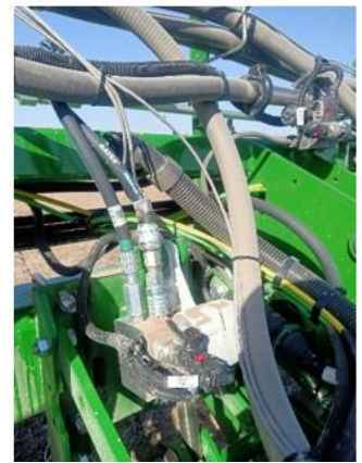
Figure 3.6. DAQ box mounting on the planter (left), accelerometers mounted on the row unit (middle), and hydraulic pressure transducers (right).
