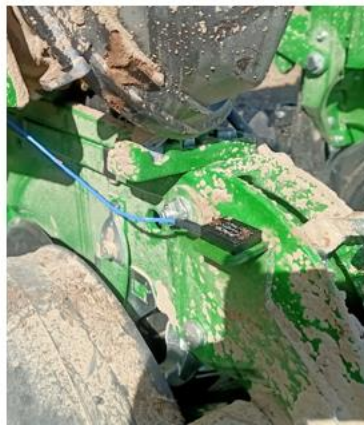
Figure 3.6. DAQ box mounting on the planter (left), accelerometers mounted on the row unit (middle), and hydraulic pressure transducers (right).
