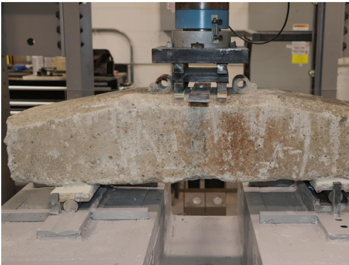
Figure 15: Tie in Rail Seat Positive Orientation
