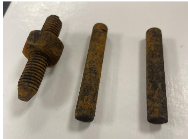
Figure 25: Corrosion at 25 Cycles
