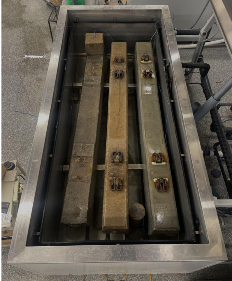
Figure 16: Railroad Ties in Freeze-Thaw Machine
