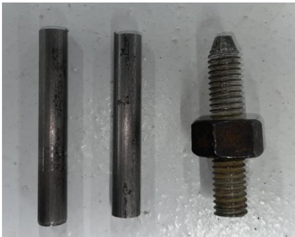
Figure 26: Corrosion at 0 Cycles
