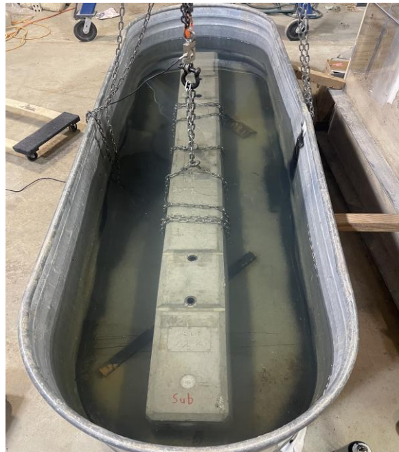
Figure 18: Post-Tensioned Tie Submerged in Water
