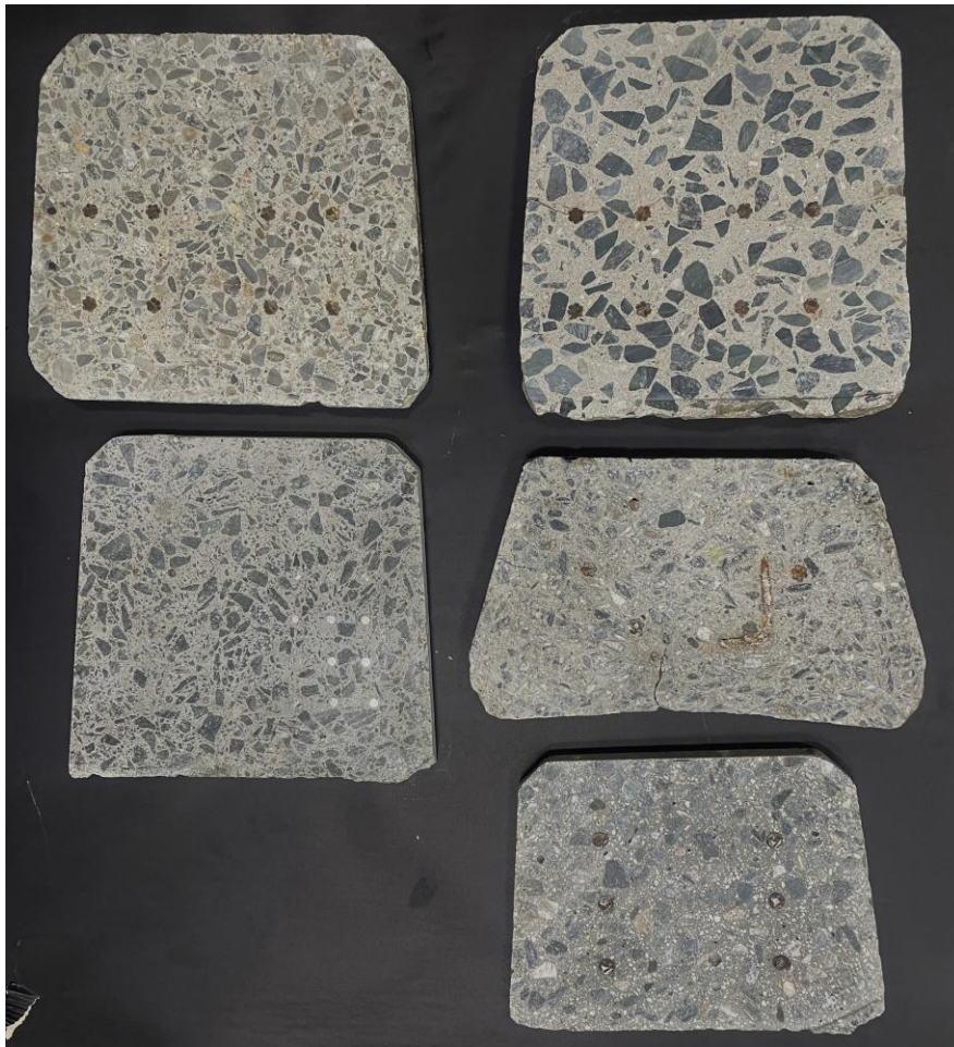
Appendix B Figure 6: All Ties Cross-Sections
