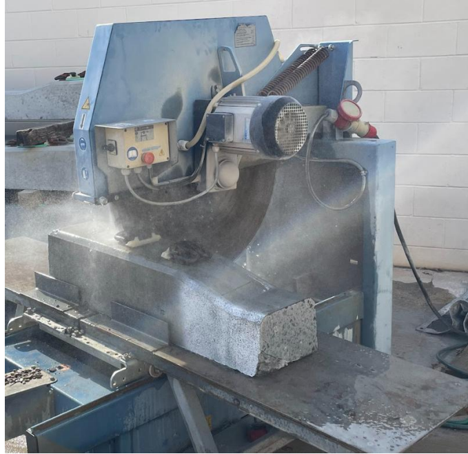
Figure 3: Dissecting Ties With the Diamond Tip Saw
