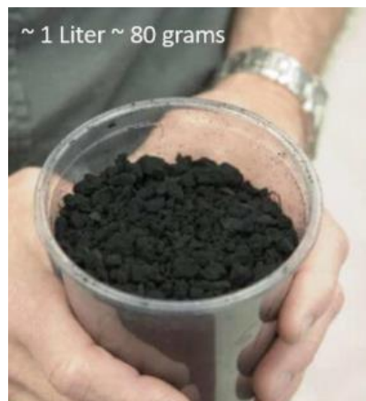
Figure 2-1 Explosion-graphene (O/C ratio = 0.3). Photo taken by Justin Wright.
