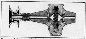
The rear axle is designed for heavy duty. It is equipped throughout with large roller bearings, adding to its life and reducing friction.
