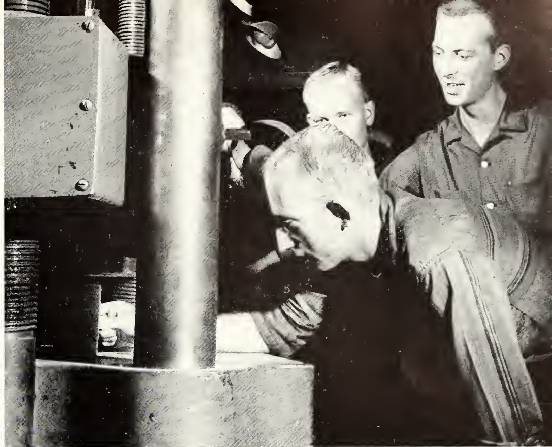
AFTER MAKING A CEMENT CYLINDER in applied mechanics, a student crushes it to test the breaking strength.
