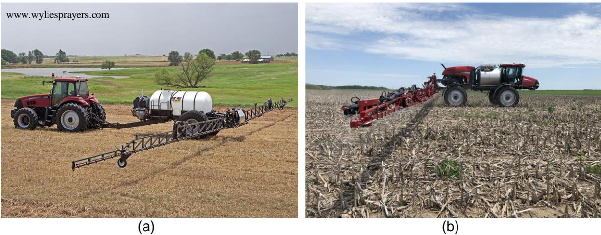
Figure 1.2. Pulled-Type (a) and Self-Propelled (b) Agricultural Sprayer.
