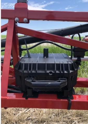
Figure 4.5. Auxiliary GNSS Receiver (B110) Located Right Next to Nozzle 16.
