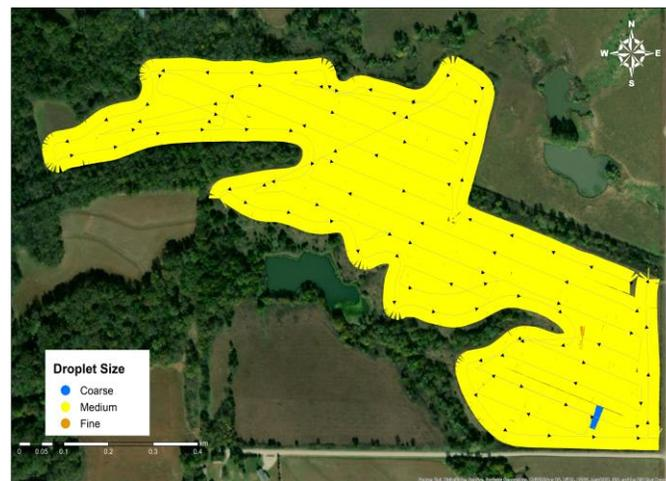
Figure 3.16. Droplet Size Spectra Uniformity Map when Using a Nozzle Tip with a Wide Range of Application Pressure to Provide the Target Droplet Size.
