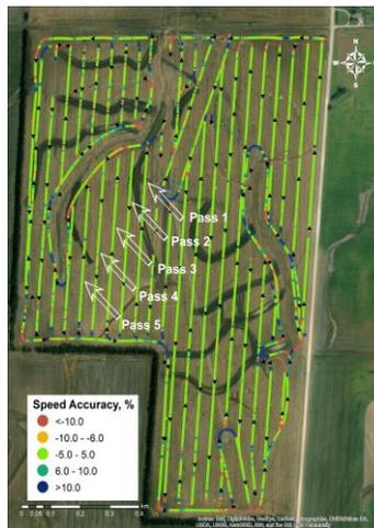
Figure 4.7. Speed Accuracy map in Field 1 Considering the Difference in Speed During Straight Passes Between the GPS 1 and GPS 2.
