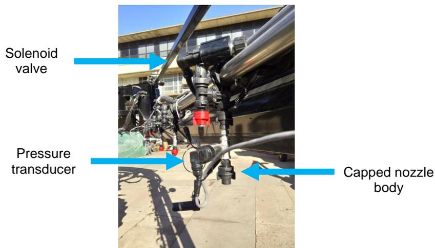
Figure 3.3. Capped Nozzle Body with the Solenoid Valve Removed to Measure Real-Time Boom Pressure.
