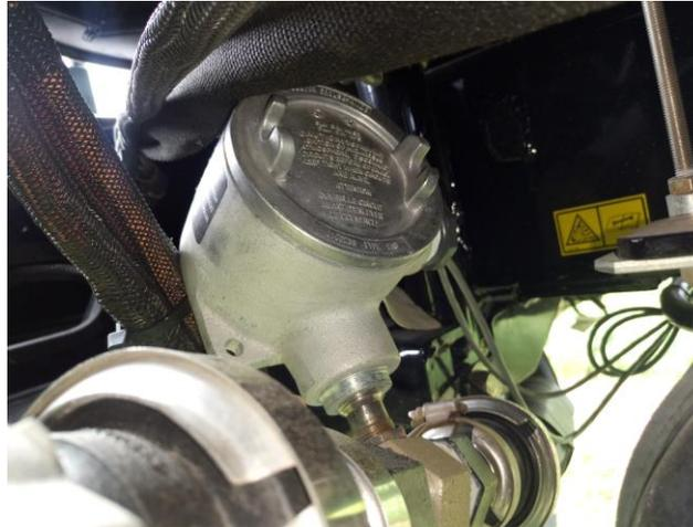
Figure 3.4. The flowmeter Used to Measure the System Flow Rate.
