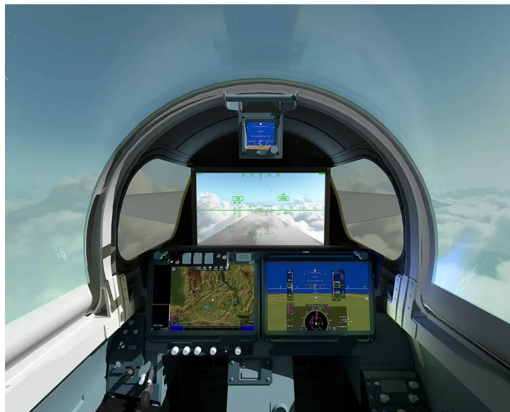
Figure 8. NASA X-59 External Vision System (NASA, 2019)
