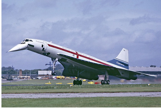
Figure 7. Concorde with Drooping Nose (Fitzgerald, 1974)
