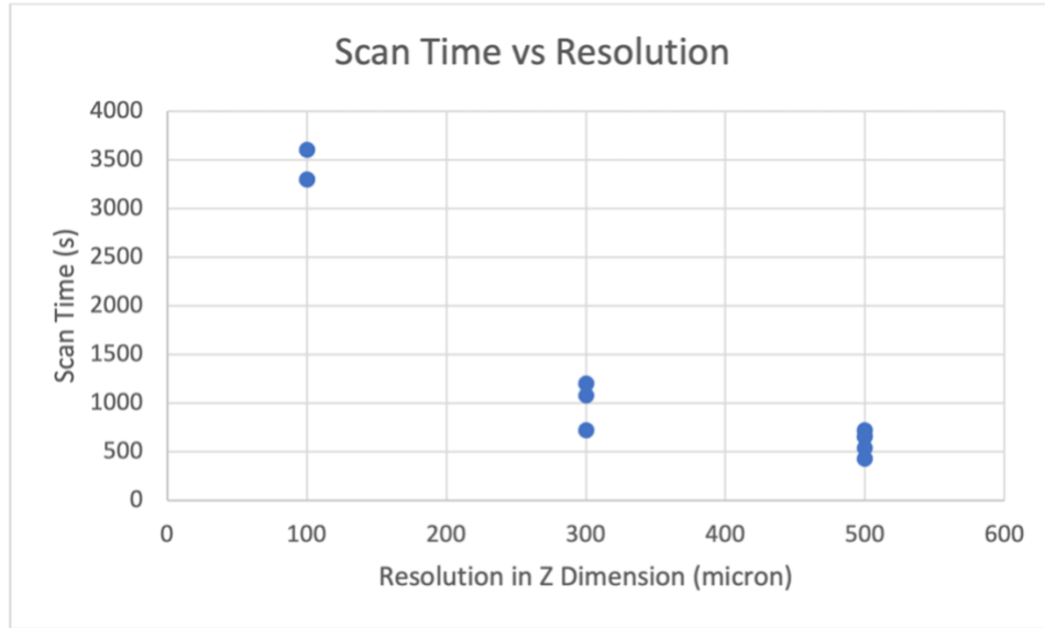
Figure 4.1: Scan time in seconds versus resolution increases in the z dimension. Resolution in x and y dimension was kept consistent at 100 microns for all samples. Images with six diffusion directions and comparable slice packages for each resolution were chosen for comparison.
