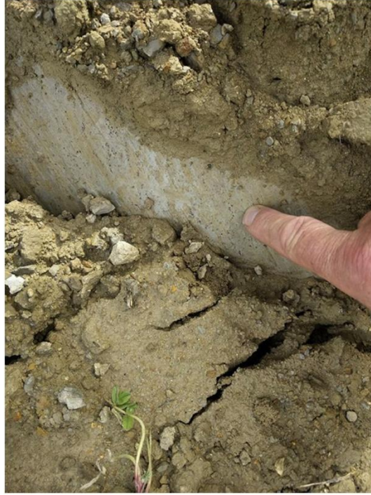
Figure 5.2: Smeared soil surface at the scarp of the landslides in Collazzone (Samia et al. 2017b)
