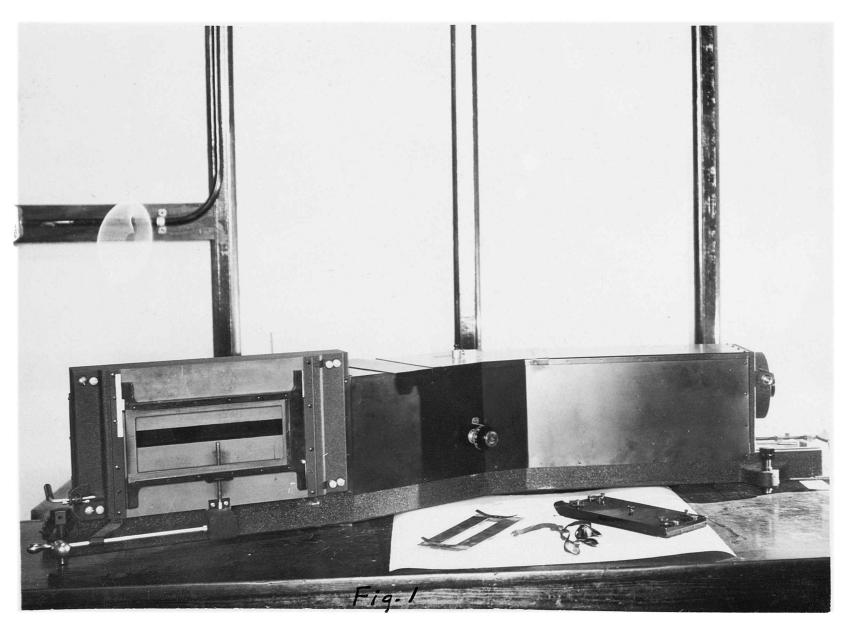
Any spectrograph is composed of the following essential parts: (1) the slit, (2) the collimator lens system, (3) the dispersing system, and (4) the recording system.
