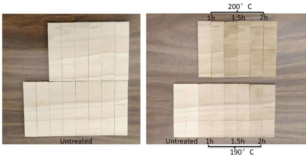
Figure 3.6 Wood color change induced by heat treatment. Longer treatment time and higher temperature induced darker colors.
