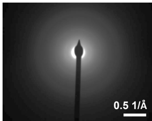
Figure A.24. SAED image of electrodeposited Li on individual VACNF fibers corresponding to Figure 2.3c.
