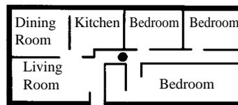
In a floor plan with only one sleeping area, place the smoke detector between the sleeping area and the rest of the house. Another detector near the rear bedrooms would offer more protection.
