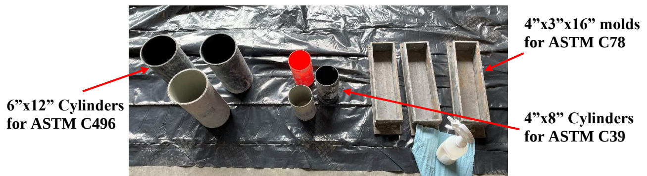
Figure 3-7: Concrete Molds for Hardened Concrete Testing
