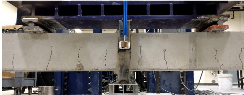
30% replacement beam #1 just after first crack
