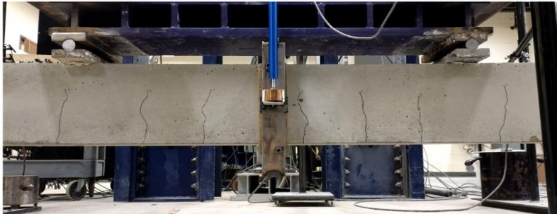
Control beam #3 just after first crack
