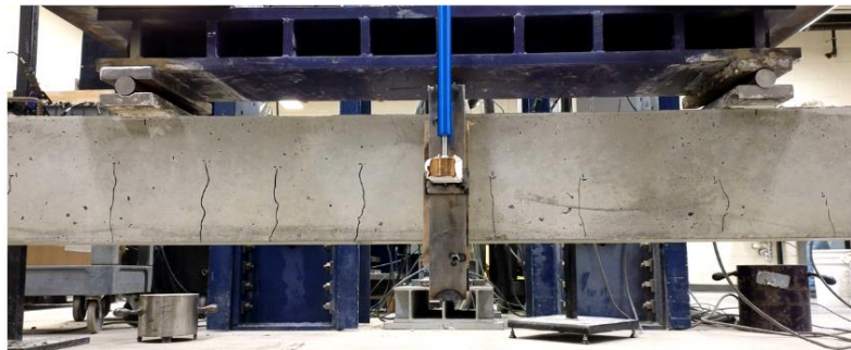
15% replacement beam #3 just after first crack
