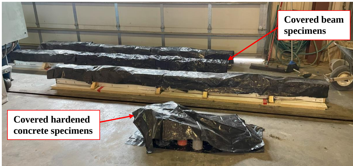
Figure 3-8: Curing of Samples
