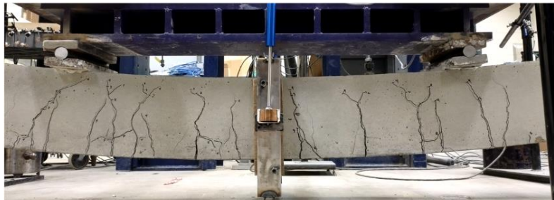
Control beam #3 at peak load
