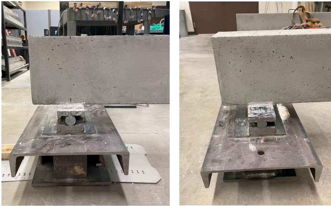
Figure 3-17: Support Conditions (Right: Pin, Left: Roller)
