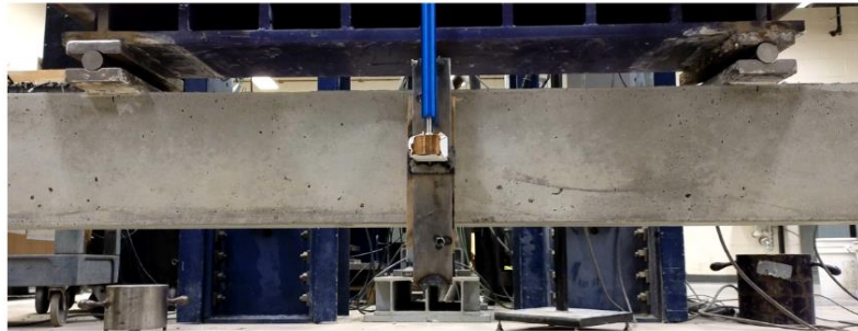
15% replacement beam #3 prior to loading
