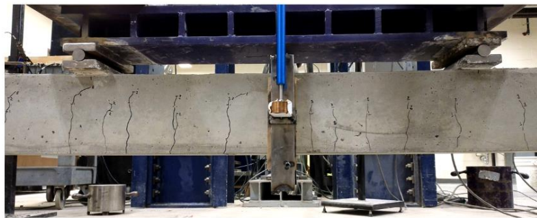
15% replacement beam #3 at reinforcement yield
