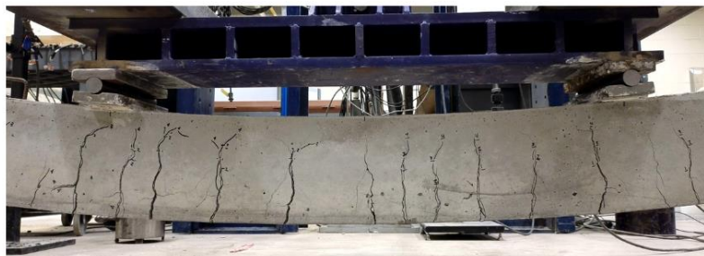
15% replacement beam #3 at peak load
