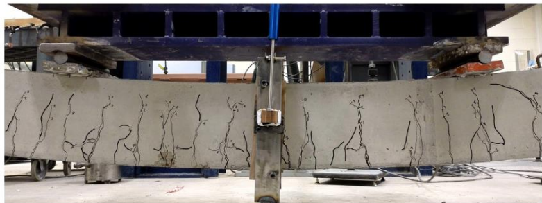
30% replacement beam #1 at peak load
