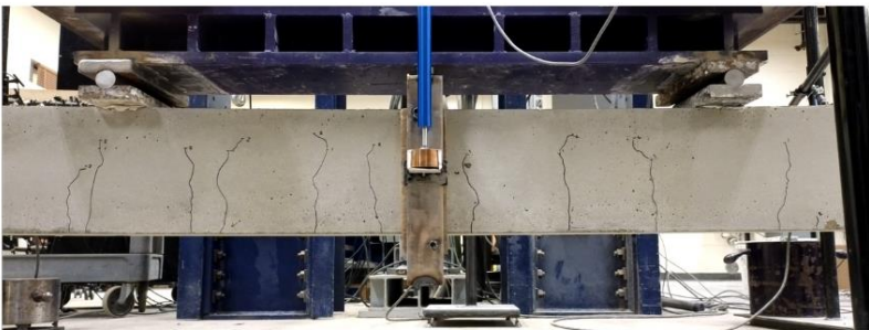
Control beam #3 at reinforcement yield
