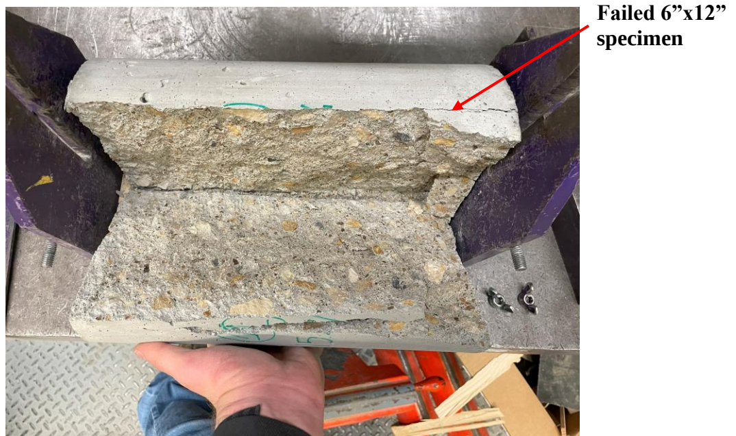
Figure 3-12: Tensile Splitting Failure
