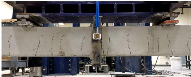
30% replacement beam #1 at reinforcement yield
