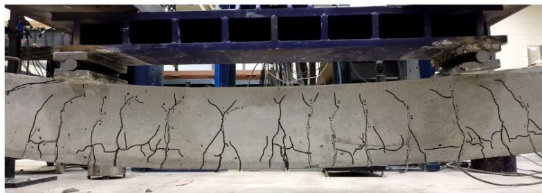
Figure 4-10: 15% Replacement Beam Crack Propagation at Each Stage of Loading
