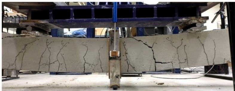
Figure 4-5: Control Beam Crack Propagation at Each Stage of Loading
