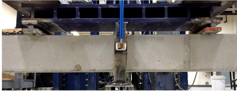
30% replacement beam #1 prior to loading
