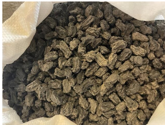
Figure 3-1: Plazrok (Coarse Aggregate Replacement)
