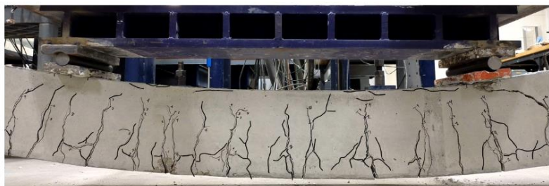
Figure 4-15: 30% Replacement Beam Crack Propagation at Each Stage of Loading
