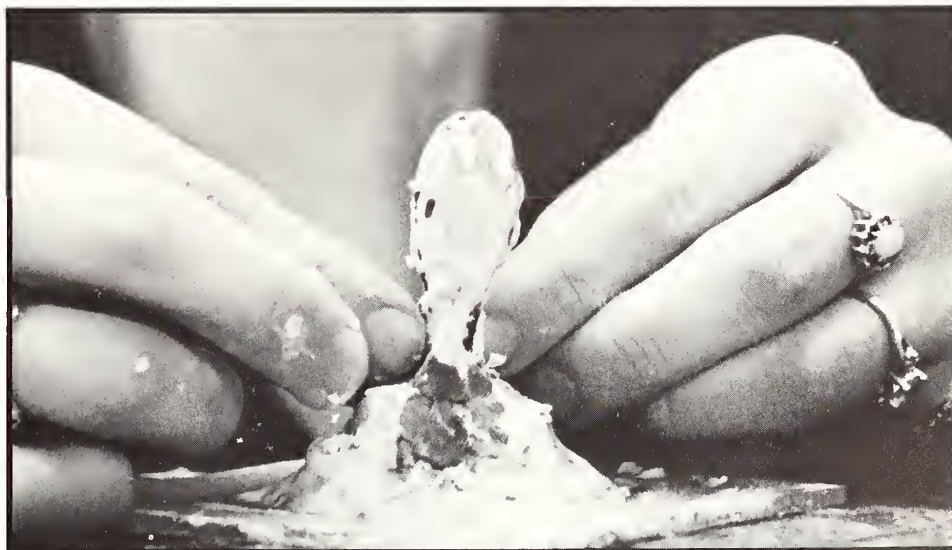
A WAX ring is prepared for making a mold by placing it on a spruce and then coating it with plaster. (Photo by Dave Watson)
