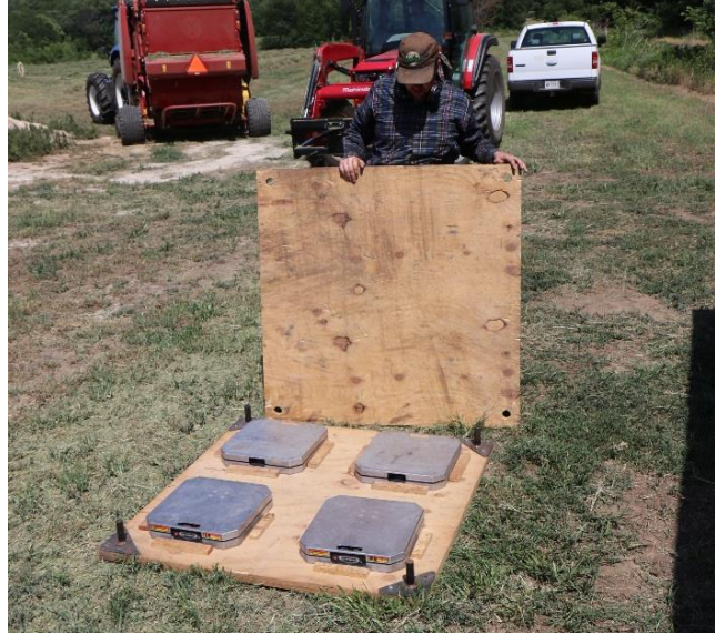
Figure 3.10: Custom Built Scale Platform with Longacre Wireless Scales
