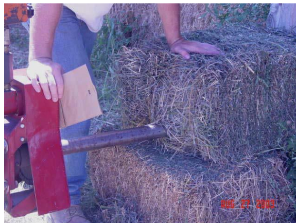
Figure 2.4: Hydraulic Boring Device used to collect core samples by Behringer (2004)
