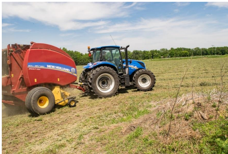
Figure 3.9: New Holland T6.180 baling alfalfa hay with New Holland RB560 Round Baler
