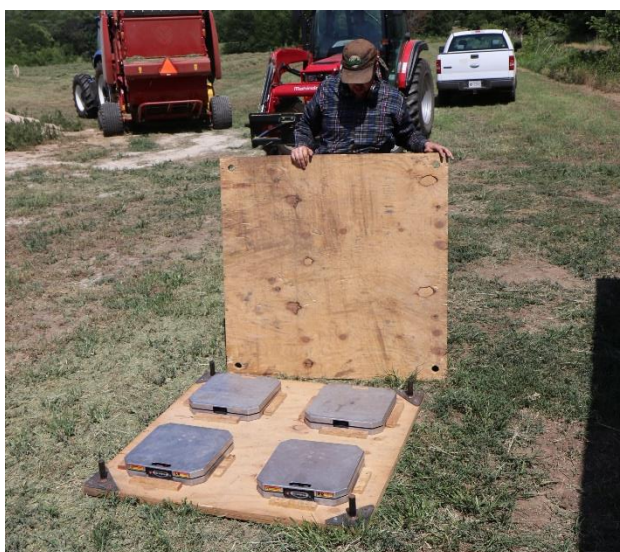
Figure 2.6: Custom Built Scale Platform with Longacre Wireless Scales
