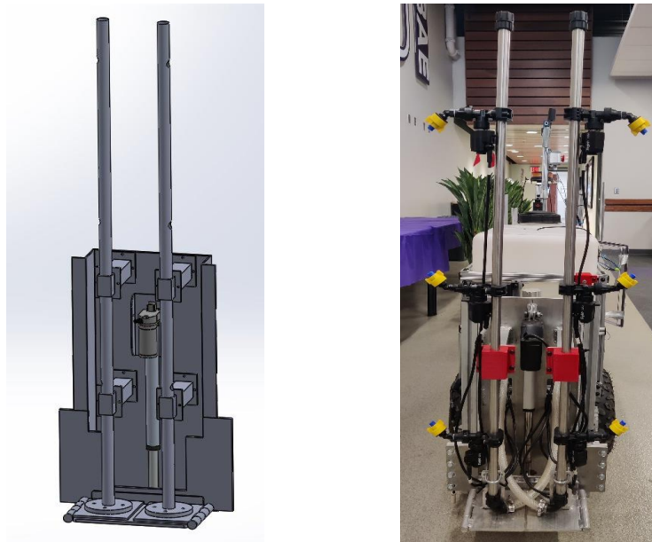
Figure 2.3 CAD Design (Left) and Real Boom Mount on Under Canopy Rover (Right)
