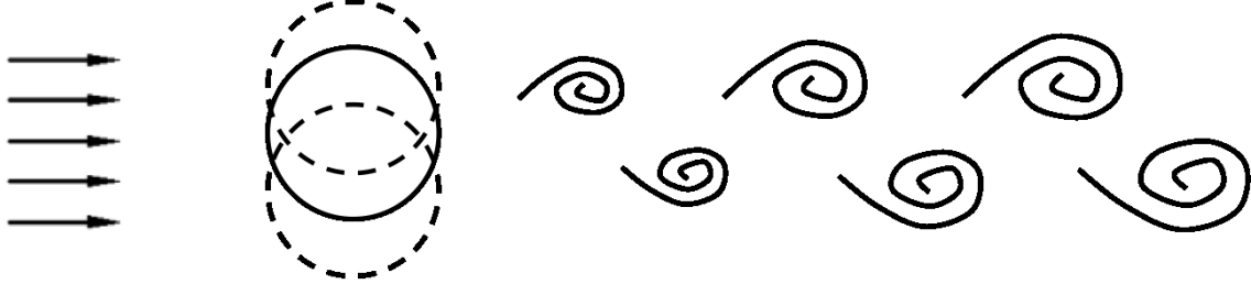
Figure 2.1: A schematic of flow passing an oscillatory cylinder.
