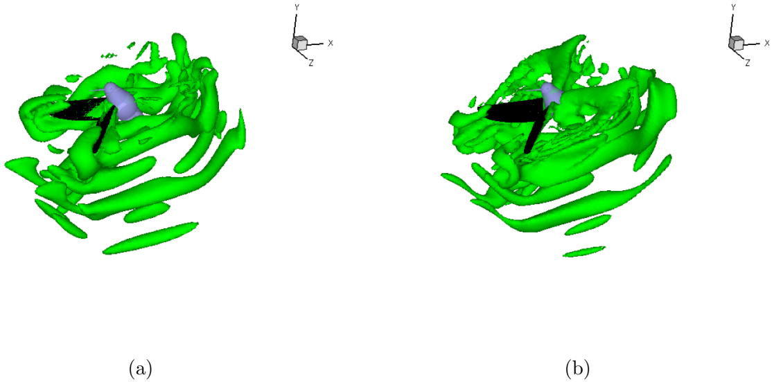
Figure 2.24: Comparison of flow field by iso-contour of Q-criterion after four periods of simulation/prediction of DNS, rebuilt result by (a) global POD coefficients computed by DNS and (b) global ROM with continuous solid domain.
