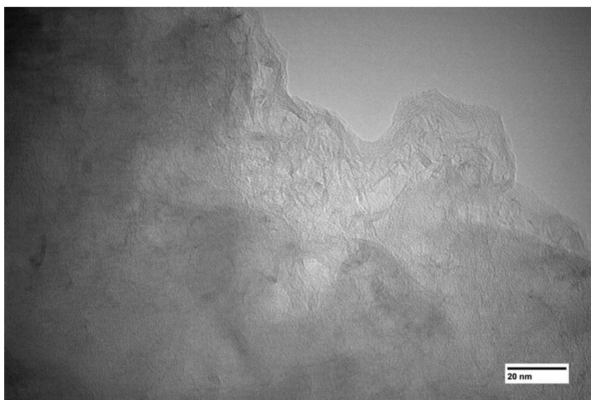
Figure A43. TEM (200 KeV) of explosion graphene-based nanobiosensor for Matrix Neutrophil Elastase Activity Detection, batch 2.
