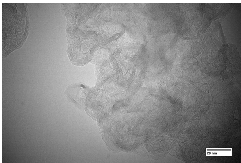
Figure A31. TEM (200 KeV) of explosion graphene-based nanobiosensor for CTSK Activity Detection, batch 2.
