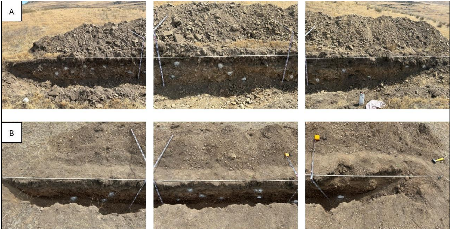
Figure 2.7: (A) Image of southern trench at WCP (Trench #2) excavated ~3 m wide and ~0.5 m deep. (B) Image of the trench opened at BGR ~5.5 m wide and ~0.5 m deep. Cobble samples were marked with white spray paint, had their “up” orientation relative to the surface notated, and then had their position horizontally and stratigraphically notated. Sediment samples had their positions notated in the trench and collected in black opaque bags to limit light exposure.
