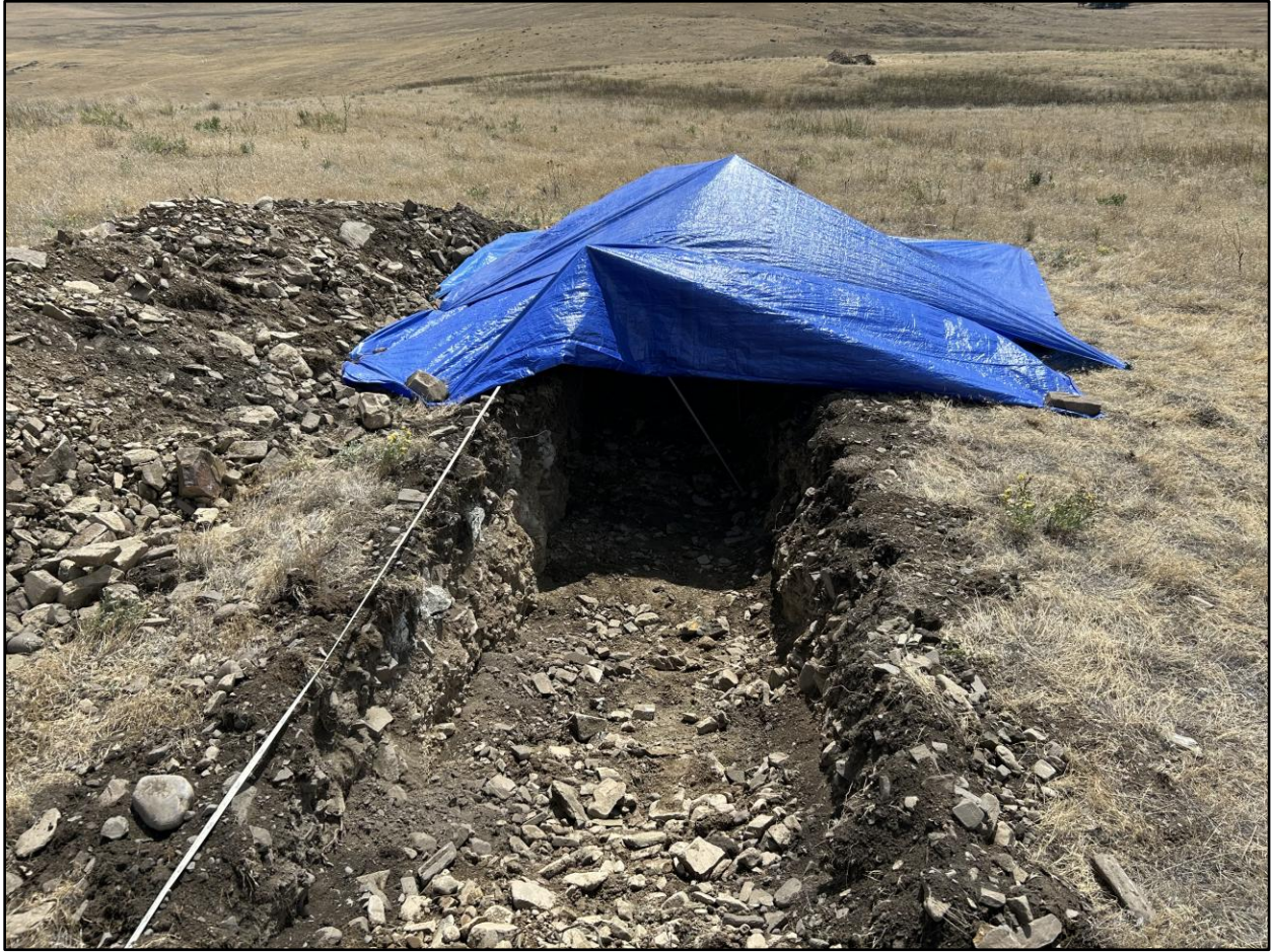
Figure 2.6: Image of the sampling setup located at WCP. It should be noted that a similar setup was used for all trenches. For each section of trench sampled from, samples were only collected from the darkest part that was covered by the tarp.
