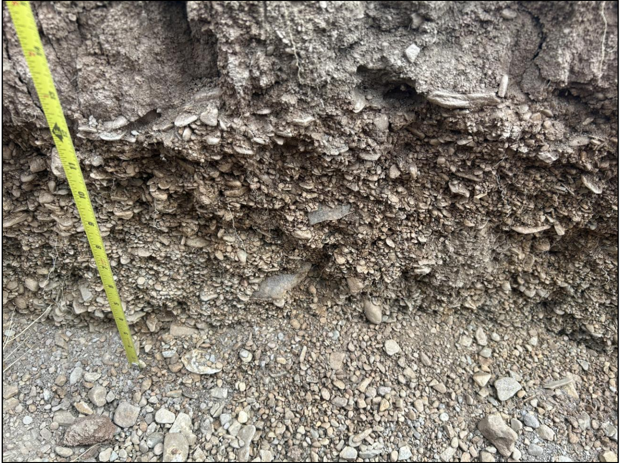
Figure 2.10: Image of matrix from the BGR trench. Clasts are much smaller compared to those found the WCP locality. The clasts found here are much rounder compared to the angular clasts found at WCP. The fabric found at this locality is mainly clast supported, indicating a higher flow velocity at this locality.
