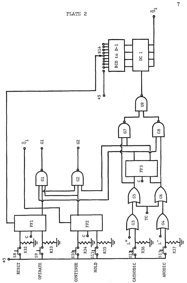
an experiment, counts the number of half cycles, and finally, resets the instrument to a prescribed set of initial conditions after the electrochemical experiment has been completed. The logic elements are all DTL and TTL integrated circuits where a logical "1" corresponds to +5V and a logical "0" corresponds to 0V.
