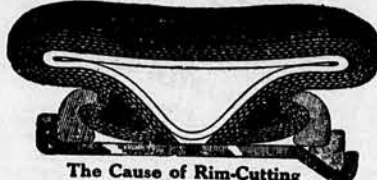
The Cause of Rim-Cutting
