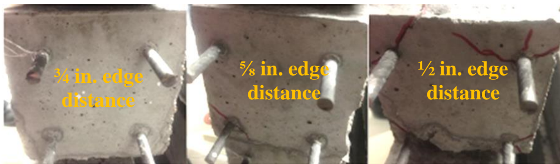
Figure 10-153: Mix#2, 6000 psi, WI-Observed Cracking (Dead End)
