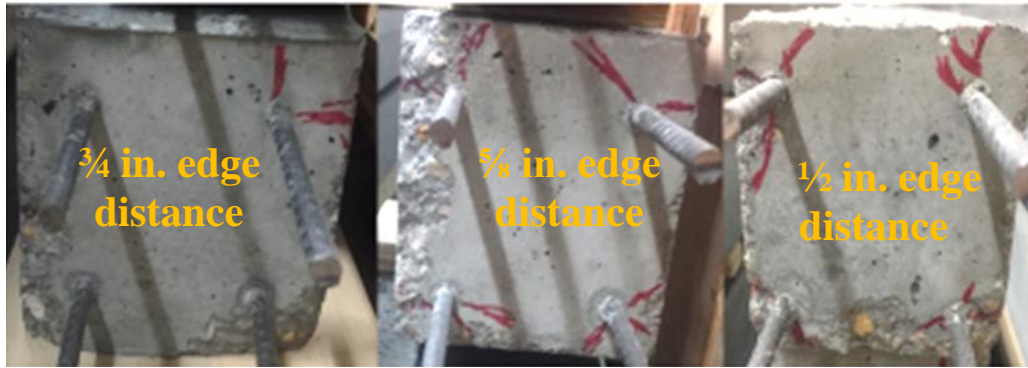
Figure 10-86: Mix#1, 4500 psi, WP-Observed Cracking (Live End)
