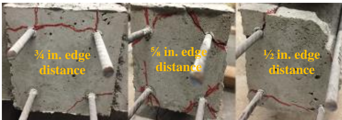
Figure 10-116: Mix#2, 6000 psi, WB-Observed Cracking (Dead End)
