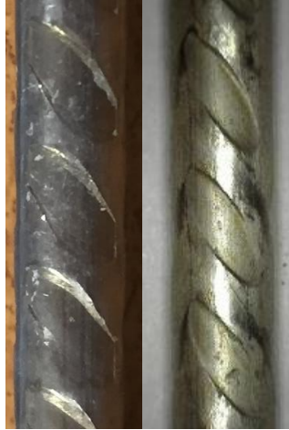
Figure 3-19: WG Wire Type Before (left) and after (right) Cleaning
