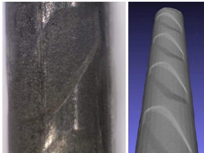
Figure 3-14: WJ Wire Type- Microscope Image and 3D Model (Haynes, 2015)
