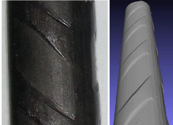
Figure 3-15: WM Wire Type- Microscope Image and 3D Model (Haynes, 2015)
