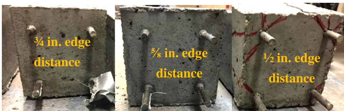
Figure 10-213: Mix#2, 6000 psi, WQ-Observed Cracking (Dead End)
