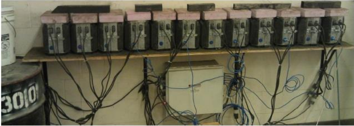
Figure 4-12: Twelve Concrete Cylinders under Temperature Control through Sure Cure Mini Controlling System
