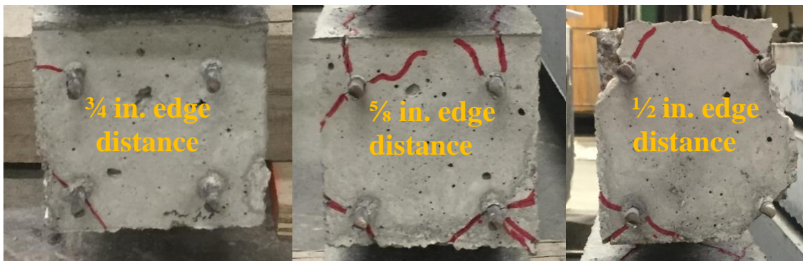
Figure 10-238: Mix#3, 4500 psi, WM-Observed Cracking (Live End)
