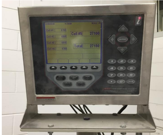
Figure 4-7: Digital Display of Prestressing Forces Measured by Load cell
