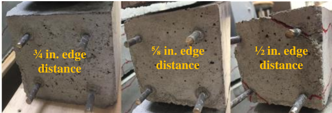
Figure 10-160: Mix#2, 4500 psi, WJ-Observed Cracking (Dead End)
