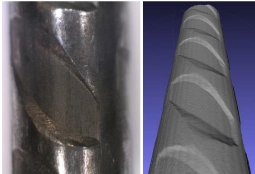
Figure 3-12: WH Wire Type-Microscope Image and 3D Model (Haynes, 2015)
