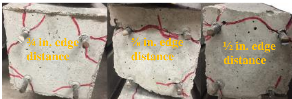
Figure 10-110: Mix#2, 4500psi, WB-Observed Cracking (Dead End)
