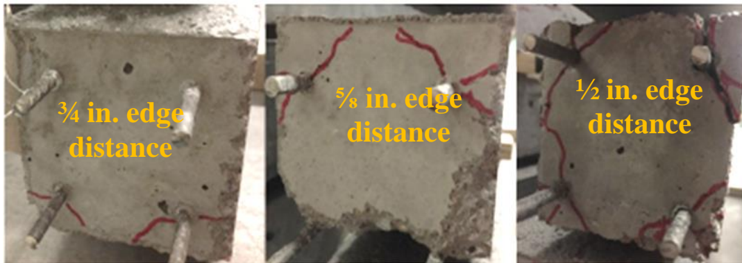
Figure 10-141: Mix#2, 4500 psi, WH-Observed Cracking (Live End)
