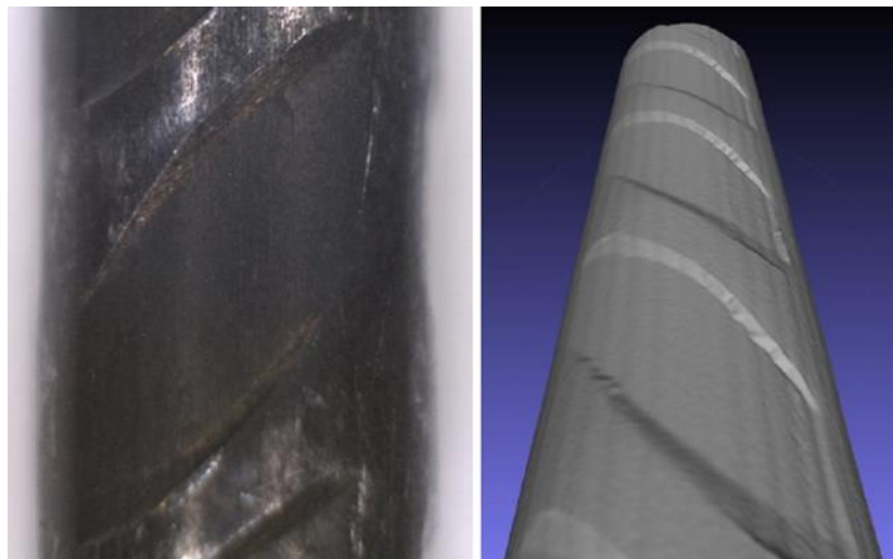
Figure 3-8: WB Wire Type- Microscope Image and 3D Model (Haynes, 2015)
