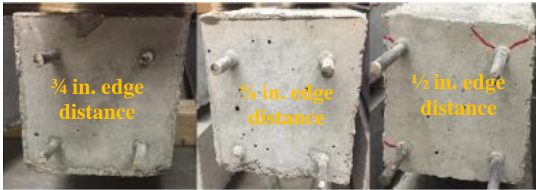
Figure 10-135: Mix#2, 4500 psi, WG-Observed Cracking (Dead End)
