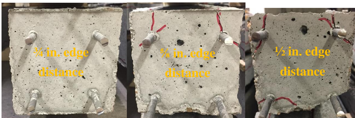
Figure 10-228: Mix#3, 4500 psi, WI-Observed Cracking (Live End)
