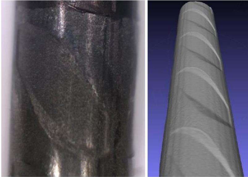
Figure 3-13: WI Wire Type- Microscope Image and 3D Model (Haynes, 2015)
