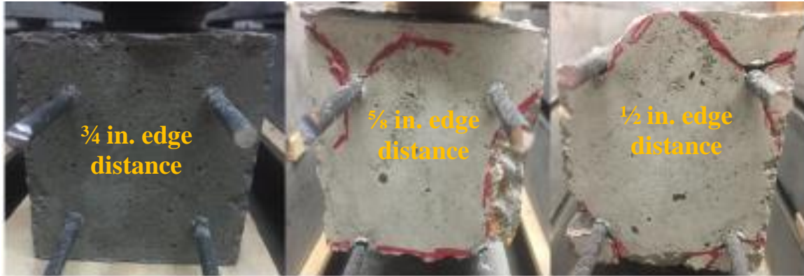
Figure 10-32: Mix#1, 6000 psi, WF-Observed Cracking (Dead End)
