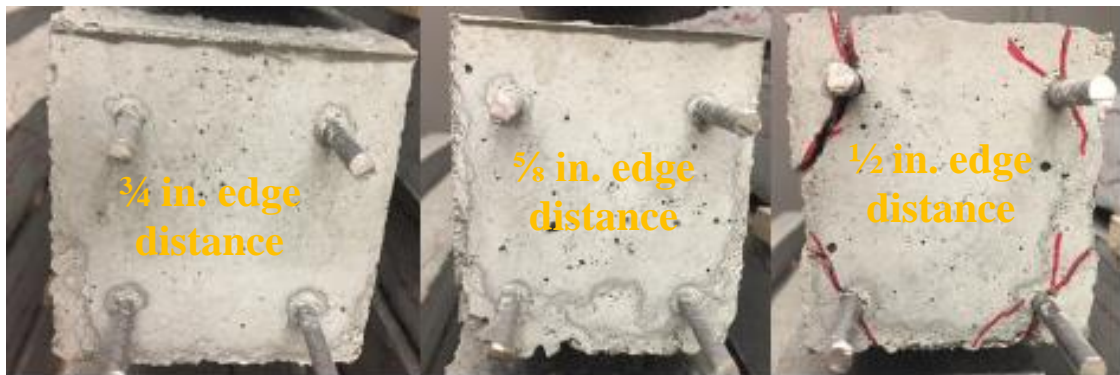
Figure 10-185: Mix#2, 6000 psi, WM-Observed Cracking (Dead End)
