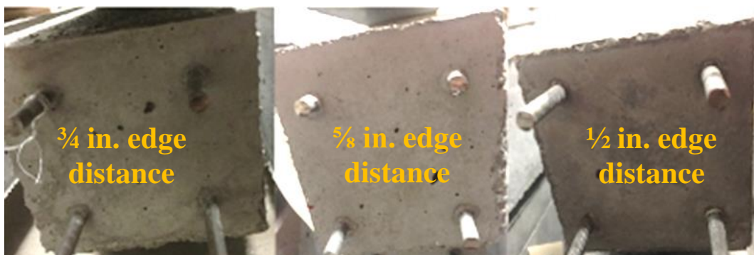
Figure 10-136: Mix#2, 4500 psi, WG-Observed Cracking (Live End)
