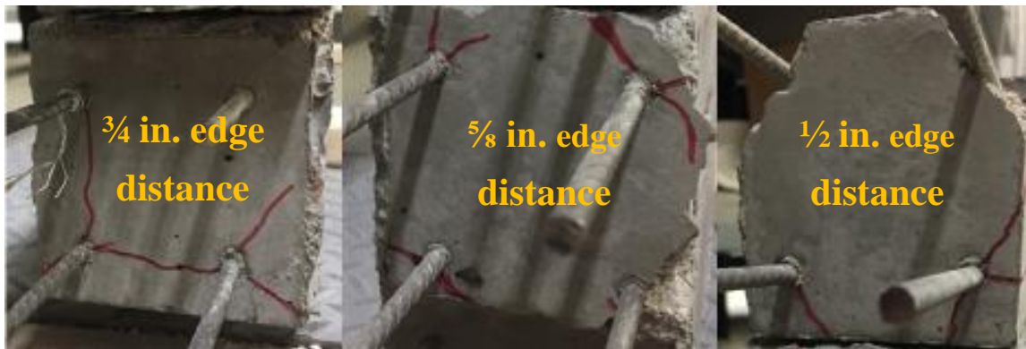
Figure 10-42: Mix#1, 4500 psi, WH-Observed Cracking (Dead End)
