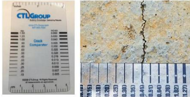
Figure 4-22: Measuring Crack Width (Savic, 2018)
