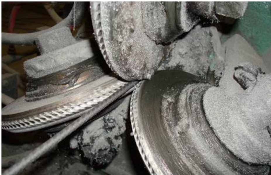
Figure 3-1: Manufacture of Indented Wire using Rollers (Beck et al., 2019)
