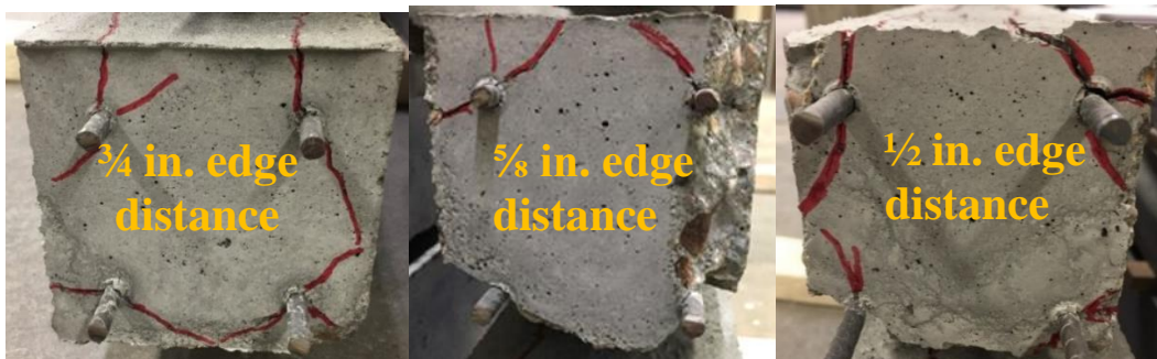
Figure 10-244: Mix#3, 4500 psi, WP-Observed Cracking (Dead End)
