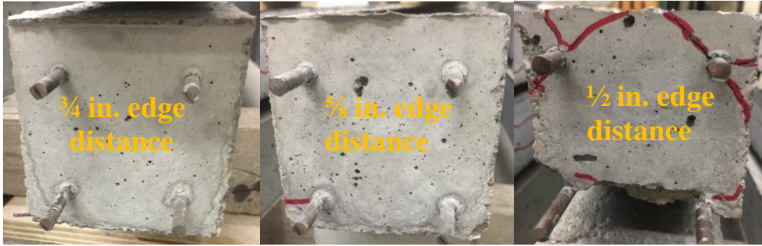
Figure 10-250: Mix#3, 4500 psi, WQ-Observed Cracking (Live End)
