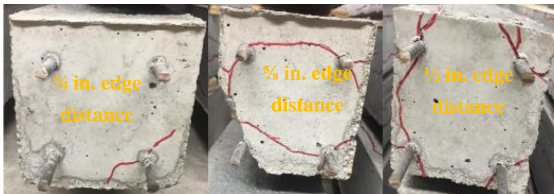
Figure 10-198: Mix#2, 6000 psi, WP-Observed Cracking (Live End)
