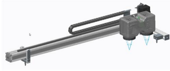
Figure 4-17: Laser Speckle Imaging System (Beck, 2010)
