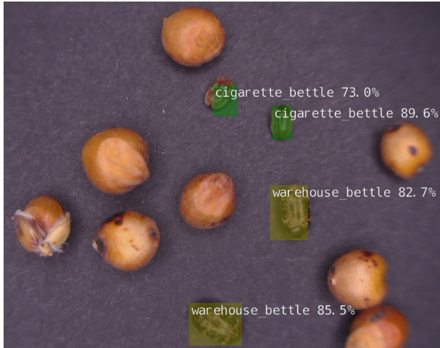
Figure 14. Live detection and identification with different grains in the background.
