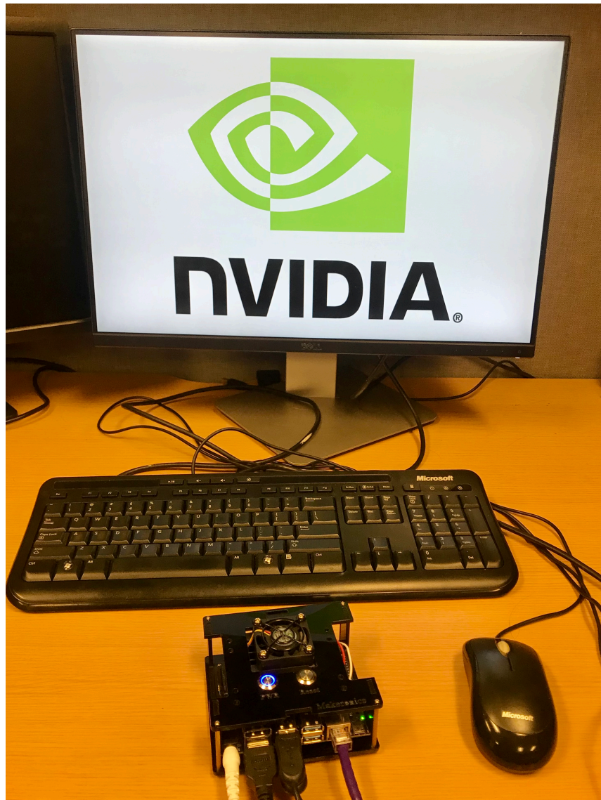
Figure 3. Jetson Nano connected to a mouse, keyboard and monitor for initial set-up.
