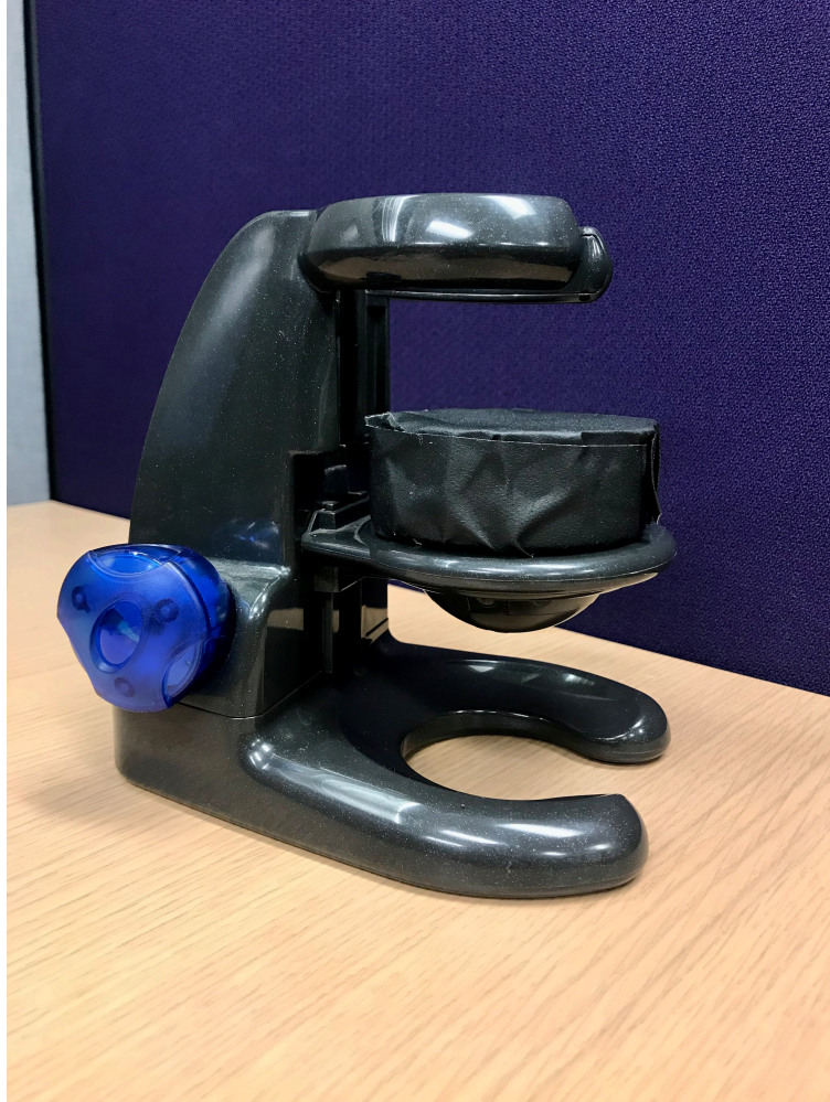
Figure 6. Microscope stand with Petri dish covered with black tape.
