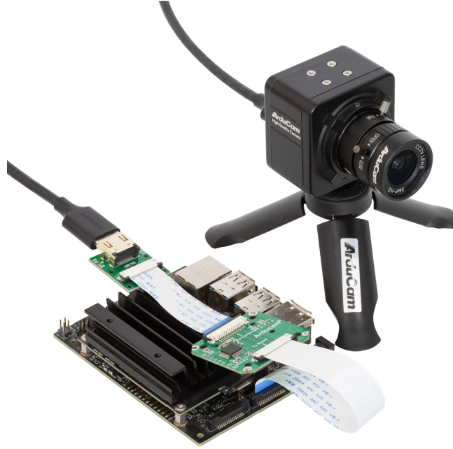
Figure 5. Arducam IMX477 [27] connected to a Jetson Nano.
