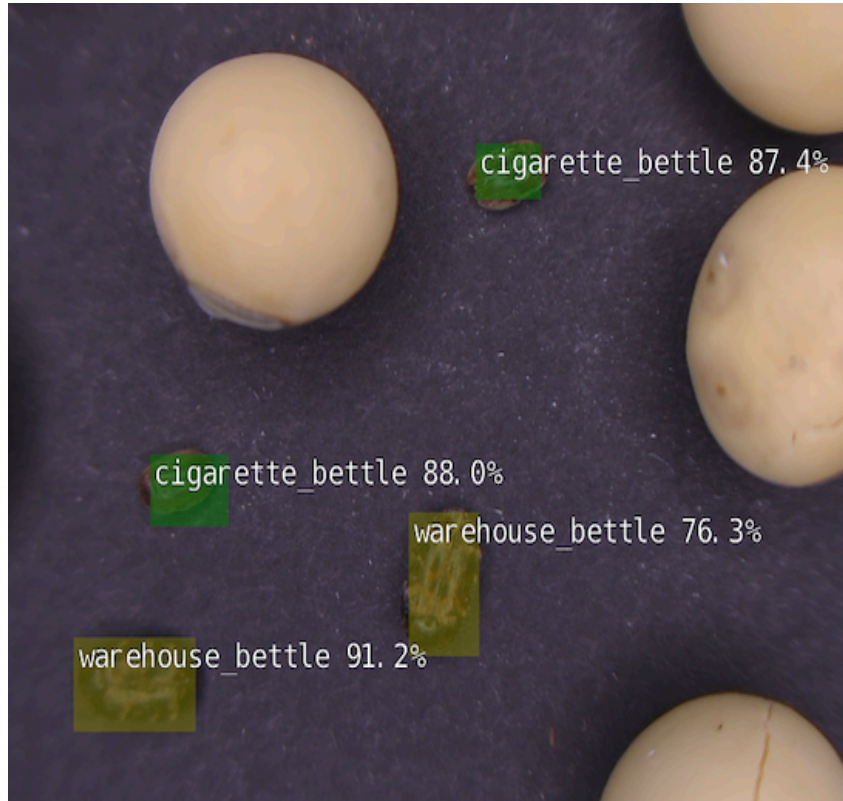
Figure 13. Live detection and identification with different grains in the background.
