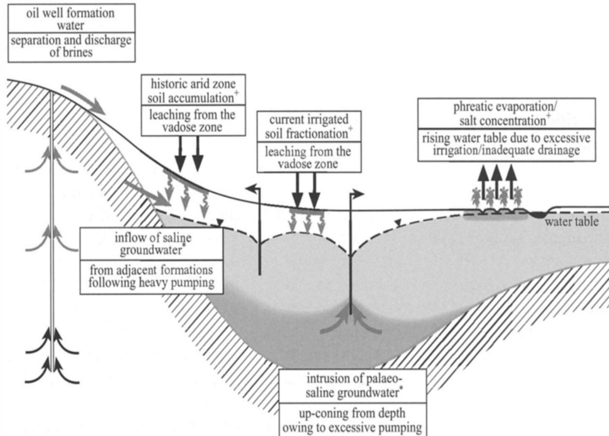
**Figure 3.2.** Saline water inflow and a subsurface drainage process
