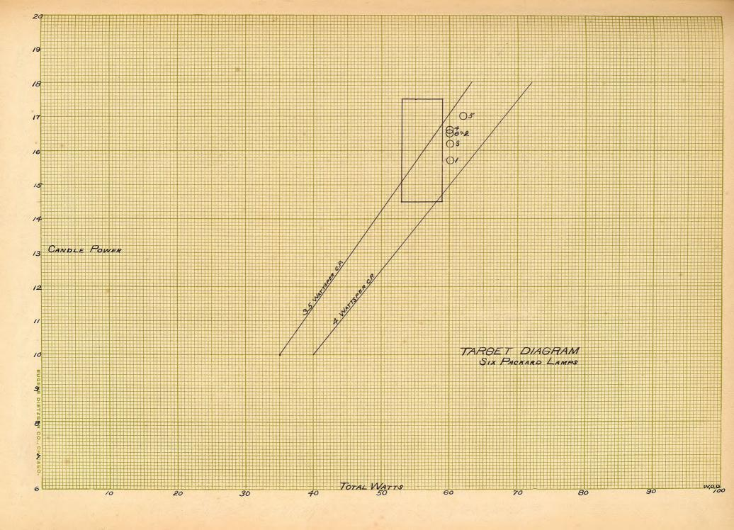
watts at the marked voltage were noted and then plotted on the diagram by placing a circle at the intersection of the horizontal candle power line and the vertical watt line corresponding to the readings. Poor marksmanship in lamp manufacture is thus clearly brought out.
