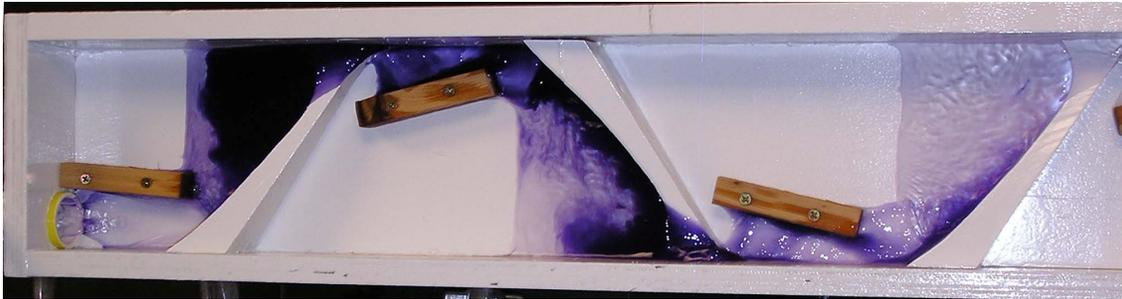
As can be seen from the purple dye pulse tracer, vortices are formed in each section of the flume. The strength of a vortex is proportional to the velocity of the fluid. The higher flow rates provide stronger vortices; however, the increase in flow rate also reduces the overall residence time of the system in which the reaction(s) occurs.
