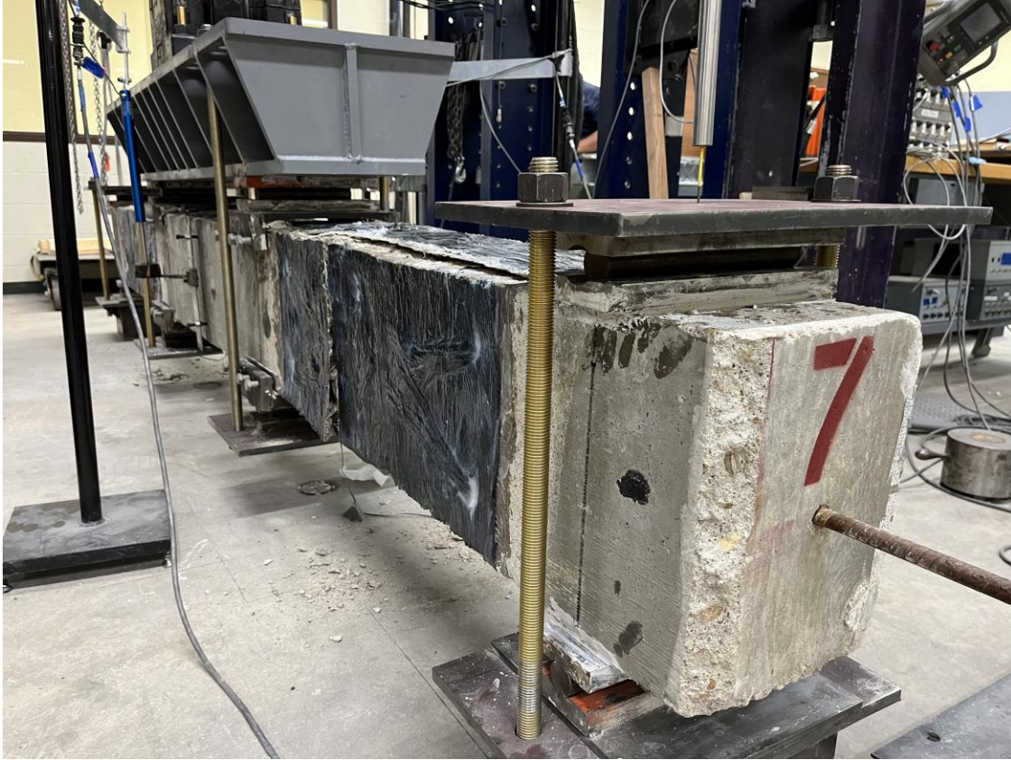
Figure 5.20. Specimen No.7 after failure
