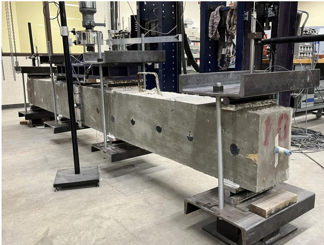
Figure 5.21. Test setup of beam No.10 before testing
