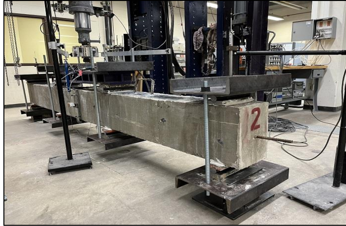
Figure 2.9. Standard testing set-up of beam No.2
