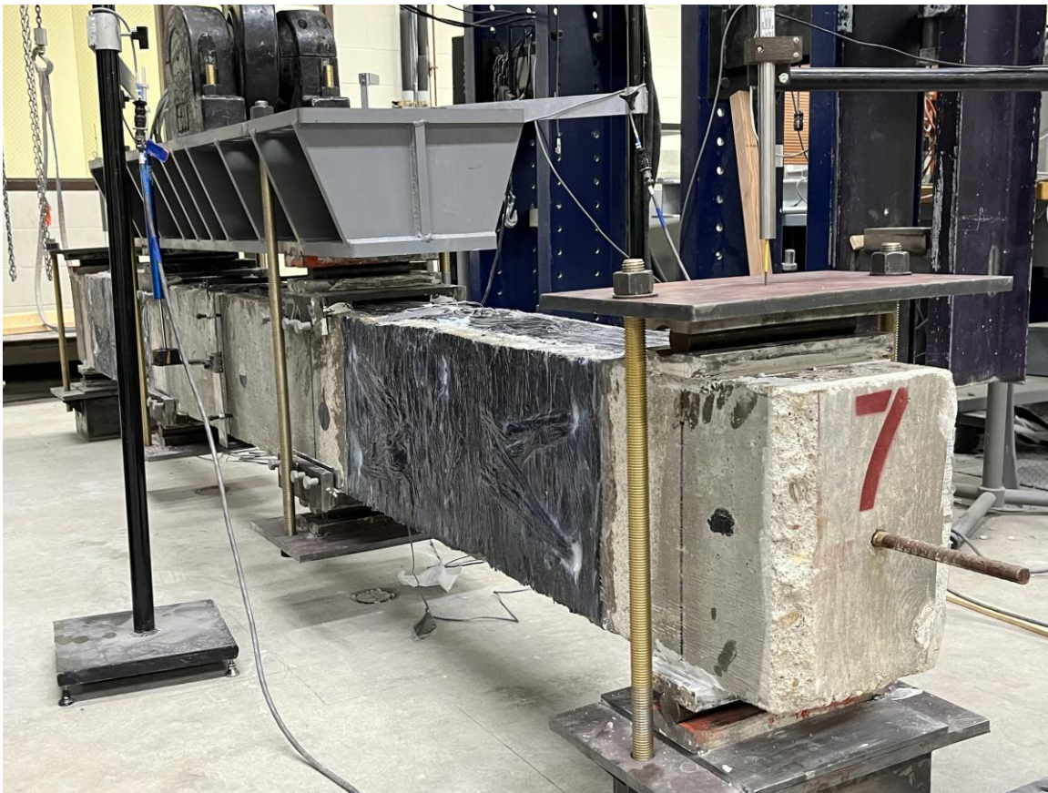
Figure 5.19. Test setup of beam No.7 before testing
