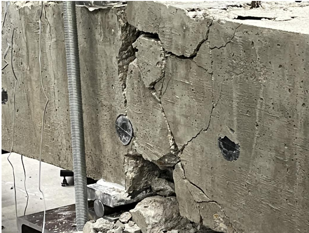
Figure 5.23. Specimen No.10 after failure
