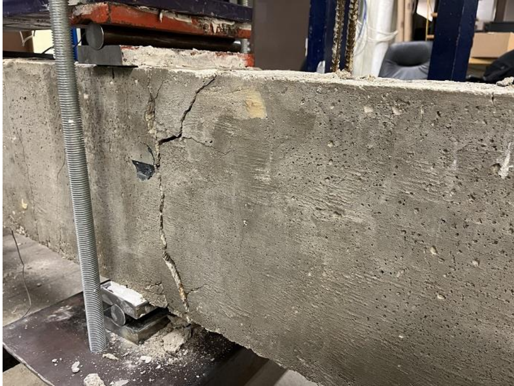
Figure 5.14. Specimen No.1 at failure.
