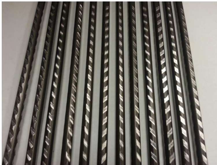
Figure 7.17: Picture of Wires With Machined Indents
