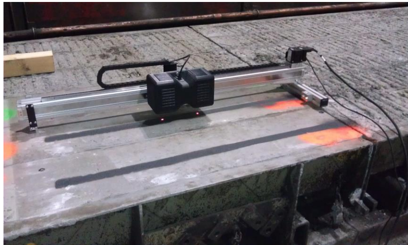
Figure 5.8: Automated LSI System on Concrete Ties in Plant
