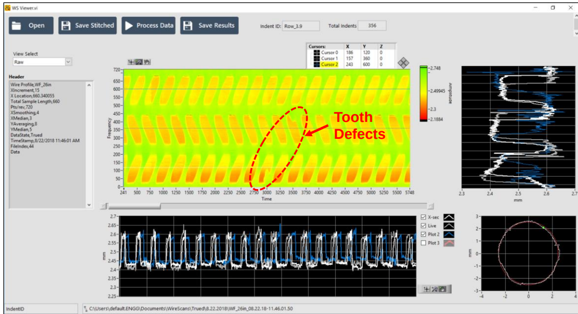
Figure 9.2: Defects Near Beginning of Scan
