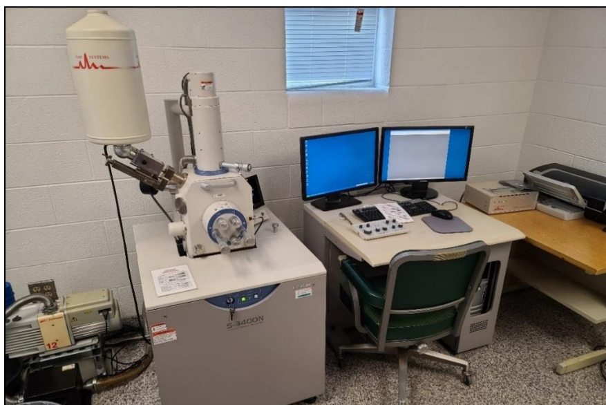
Fig. 4-10. Image of the Hitachi S-3400N SEM with coupled XRF analysis system.
