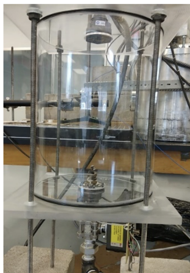
Figure 7.2: (a) 17 L transparent chamber for viewing dispersion, (b) schematic of the explosion set up in a 17 L aluminum chamber.
