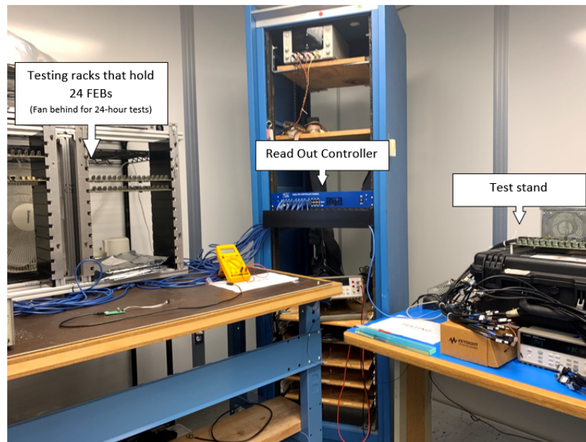
Figure 5.1: Front End Board testing setup at K-State
