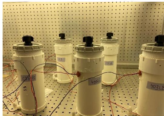
**Figure S4.3. PVC column design: Right figure shows sealing achieved by using lids (having septa on top) to cover/seal the top properly for gas sampling, photo taken in growth chambers**
