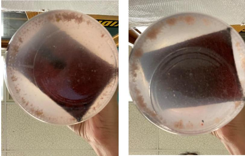
**Figure S4.2. Photo of second replicate of *Geobacter* coated electrodes, coverage on first (left) photo was considered 85%-high biofilm treatment, while on second (right) photo was considered 45%-low biofilm treatment by visual analysis**
