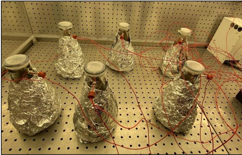
**Figure S3. 1. MFC set up using 1000-mL flasks**
